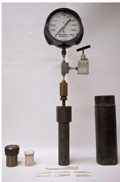
Figure 1: Technology in hydrothermal synthesis (from left): stainless steel acid digestion vessel with PTFE liner (Parr Instrument Co.), Inconel 718 Tuttle cold-seal autoclave with silver reaction ampoules, scalable to larger sizes.
