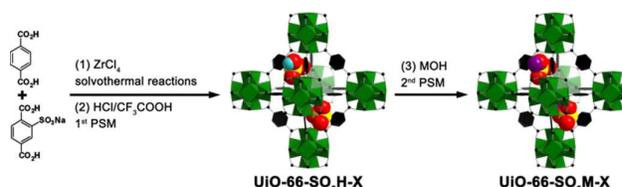
**Fig. 18** Synthesis of UiO-66-SO<sub>3</sub>M-X involving mixed ligand and post-synthetic metalation.<sup>91</sup> Reprinted with permission from John Wiley and Sons Copyright 2014.
