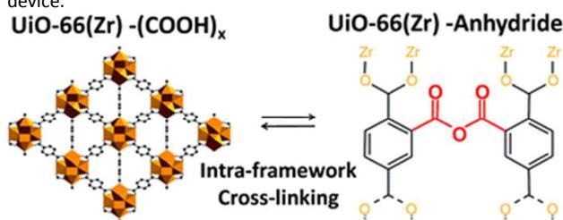
**Fig. 15** Acid-functionalized UiO-66(Zr) MOFs and their evolution after intra-framework cross-linking.<sup>185</sup> Reprinted with permission from The Royal Society of Chemistry Copyright 2015.
