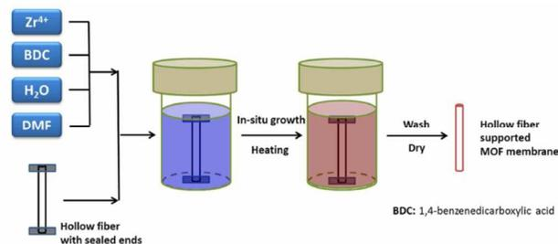
**Fig. 20** Scheme for direct preparation of pure UiO-66(Zr) membranes supported on porous ceramic hollow fibers.<sup>203</sup> Reprinted with permission from American Chemical Society Copyright 2015.
