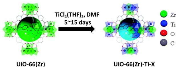
**Fig. 13** Scheme for metal cation exchange of UiO-66(Zr) with Ti(IV)
