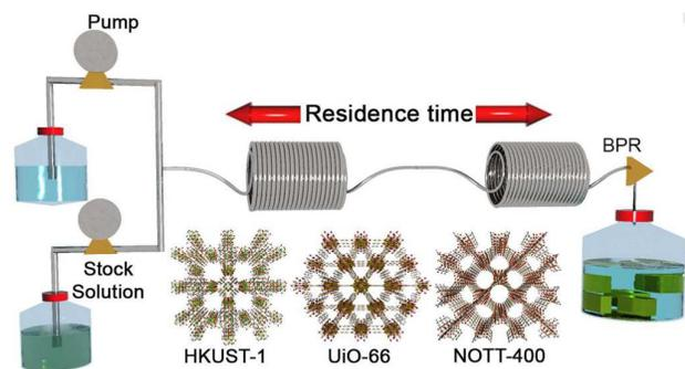
**Fig. 5** A setup of flow reactor for the continuous production of MOFs.<sup>119</sup> Reprinted with permission from Nature Publishing Group Copyright 2014.
