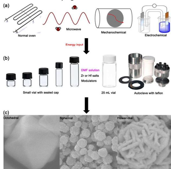
**Fig. 2** Scheme of solvothermal synthesis: (a) energy sources; (b) apparatus; (c) morphologies of MOF products.
