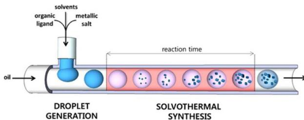
**Fig. 6** Scheme of a microchemical process for ultrafast MOF synthesis.<sup>121</sup> Reprinted with permission from American Chemical Society Copyright 2013.
