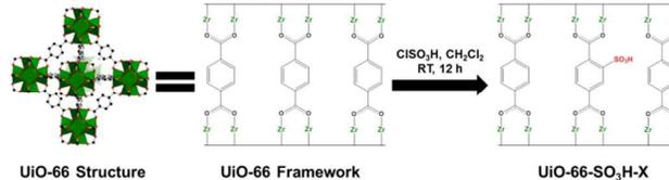
**Fig. 7** Synthetic route of UiO-66-SO<sub>3</sub>H-X.
