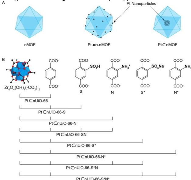
**Fig. 12** Schematic representation for the preparation of nMOF and Pt-loaded nMOFs.<sup>145</sup> Reprinted with permission from American Chemical Society Copyright 2015.
