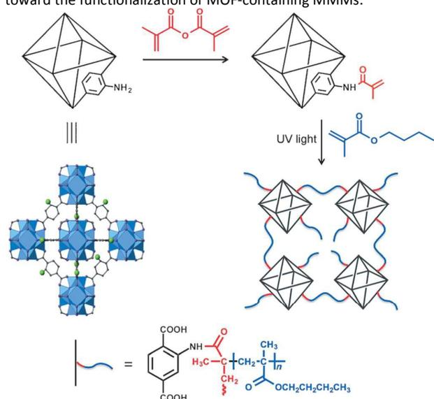
**Fig. 23** Scheme for the preparation of flexible stand-alone membranes by copolymerization of methacrylic anhydride functionalized UiO-66(Zr)-NH<sub>2</sub> nanocrystals with butyl methacrylate (BMA) under UV light irradiation.<sup>214</sup> Reprinted with permission from John Wiley and Sons Copyright 2015.
