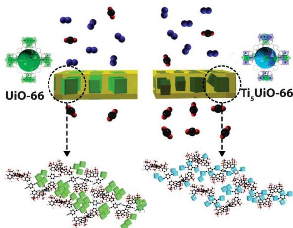
**Fig. 21** Scheme for Ti-loaded UiO-66@PIM-1 MMMs.<sup>212</sup> Reprinted with permission from Nature Publishing Group Copyright 2015.
