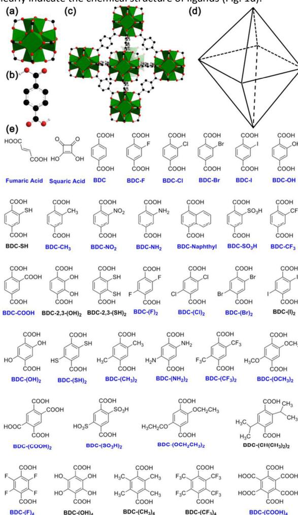
**Fig. 1** Illustration of UiO-66: (a) secondary building units (SBUs); (b) BDC ligand; (c) crystal model; (d) a simplified form; (e) commercially available or synthetically feasible BDC-type ligands. Ligands labeled as blue indicate their according MOFs have been attempted.
