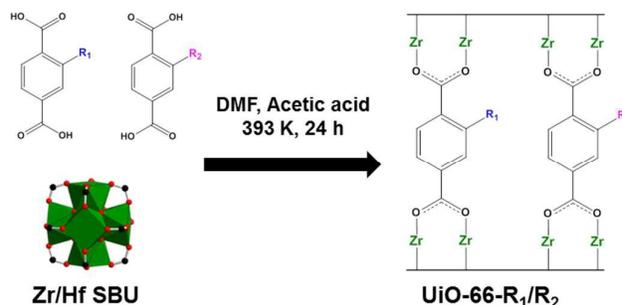
**Fig. 17** Scheme of mixed ligand approach for the synthesis of multi-functional UiO-66-type MOFs.<sup>187, 188</sup>
