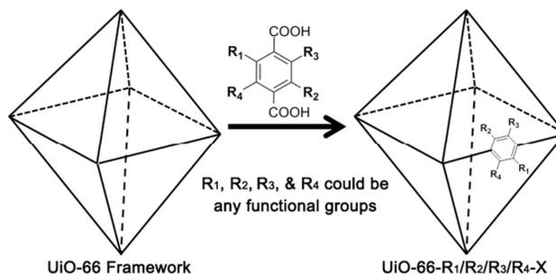
**Fig. 14** Scheme for post-synthetic ligand exchange of UiO-66-type MOFs.<sup>170, 179, 181, 183</sup>
