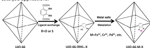
**Fig. 19** Synthesis of functional UiO-66-type MOFs involving post-synthetic ligand exchange and metalation.<sup>180, 182</sup>
