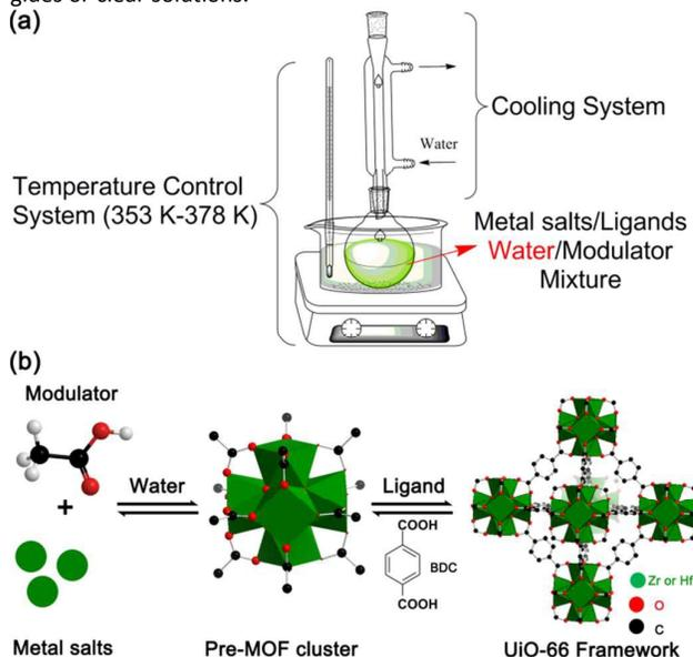
**Fig. 4** Apparatus (a) and proposed mechanism (b) of modulated hydrothermal (MHT) approach for the synthesis of UiO-66-type MOFs.<sup>102</sup>
