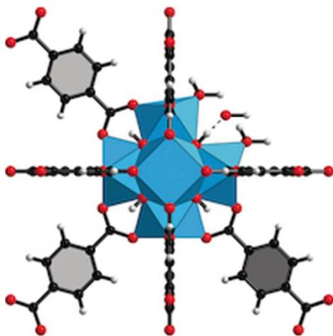
**Fig. 24** Schematic illustration of defect sites in UiO-66 single crystals. The missing BDC ligand is replaced by water molecule and overall charges are counterbalanced by hydroxide anions hydrogen bonded within the pores of the framework. Reprinted with permission from John Wiley and Sons Copyright 2015.<sup>80</sup>
