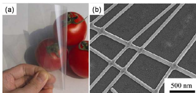
**Fig. 11** (a) Photograph of Ag nanowires deposited on a transparent PET substrate and (b) FE-SEM images of Ag NWs on a PET substrate after mechanical processing.<sup>136</sup> (Reproduced with permission from ref. 136)
