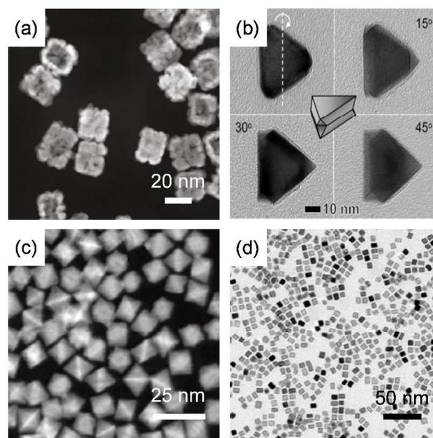
**Fig. 8** TEM images of (a) Pd-Pt nanocages,<sup>112</sup> (b) Pd-Pt triangular nanoplates,<sup>113</sup> (c) Pt-Ni octahedrons<sup>114</sup> and (d) Pt-Pd cubes.<sup>115</sup> (Figures (a), (b), (c) and (d) were reprinted with permission from ref. 112, 113, 114 and 115 correspondingly)
