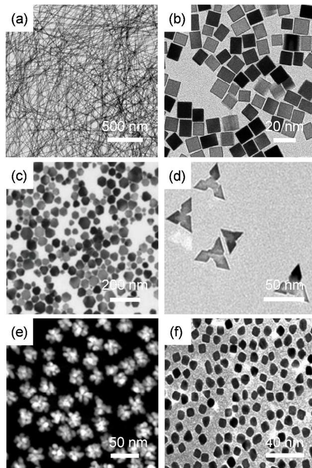
**Fig. 6** TEM images of PVP-assisted synthesized Pd nano- (a) wires,<sup>95</sup> (b) cubes,<sup>97</sup> (c) plates<sup>98</sup> and (d) arrow-headed tripods<sup>99</sup> and TEM images of PVP-assisted synthesized Pt nano (e) flowers<sup>100</sup> and (f) cubes and tetrahedra.<sup>101</sup> (Figures (a), (b), (c), (d), (e) and (f) were reproduced with permission from ref. 95, 97, 98, 99, 100 and 101 respectively)
