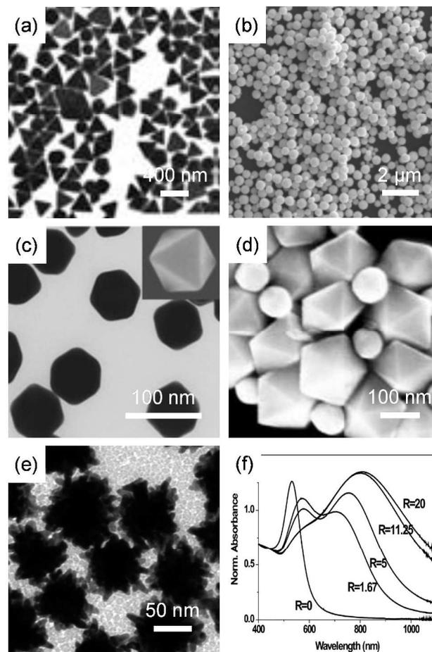
**Fig. 5** SEM/TEM images of PVP-moderated shape-controlled gold nanostructures including (a) triangular plates,<sup>31</sup> (b) spheres,<sup>77</sup> (c) octahedra,<sup>79</sup> (d) decahedra,<sup>80</sup> (e) stars<sup>81</sup> and Vis-NIR spectra (f) of gold nanostars prepared using different ratios of seeds to salt concentration.<sup>81</sup> (Figures (a), (b), (c), (d) and (e-f) were reprinted with permission from ref. 31, 77, 79, 80 and 81 correspondingly)
