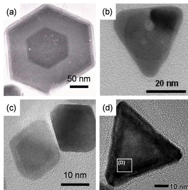
**Fig. 7** TEM images of (a) hexagonal Au@Ag,<sup>105</sup> (b) Au nanoring@Ag,<sup>107</sup> (c) polyhedral Pt@Pd<sup>110</sup> and (d) Pd@Pt triangular plates.<sup>111</sup> (Figures (a), (b), (c) and (d) were reprinted with permission from ref. 105, 107, 110 and 111 respectively)
