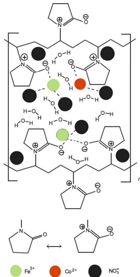
**Fig. 13** Distribution of metallic ions and nitrate in the cavities of PVP – The case of CoFe<sub>2</sub>O<sub>4</sub> NPs.<sup>150</sup> (reproduced with permission from ref. 150)
