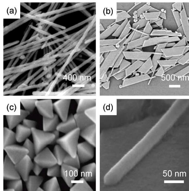
**Fig. 4** SEM images of Ag nanocrystals prepared using PVP-assisted polyol and/or DMF syntheses showing morphologies of (a) wires,<sup>60</sup> (b) flags,<sup>66</sup> (c) bipyramids,<sup>67</sup> and (d) nanobeams.<sup>68</sup> (Figures (a), (b), (c) and (d) were reproduced with permission from ref. 60, 66, 67 and 68 respectively)
