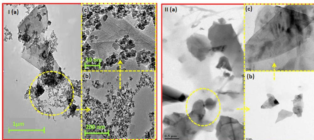
**Fig.4**HR-TEM image graphene-titanium dioxide nanocomposite (I a b and c) and graphene (II a, b and c). (See also supporting information Figure S-3 in ESI†).
