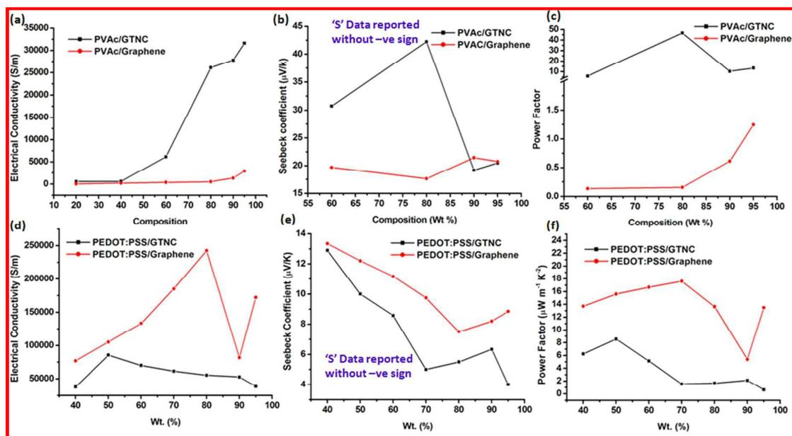
**Fig. 5** (a) electrical conductivity, (b) seebeck coefficient and (c) power factor with different filler concentration for PVAc based composite. (d) electrical conductivity, (e) seebeck coefficient and (f) power factor with different filler concentration for PEDOT:PSS based composite.
