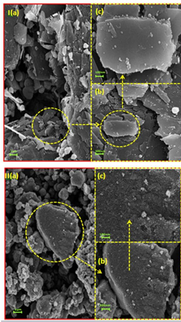
**Fig. 3** FESEM traces GTNC (I a, b and c) and nano TiO<sub>2</sub> (II a, b and c) at different magnification
