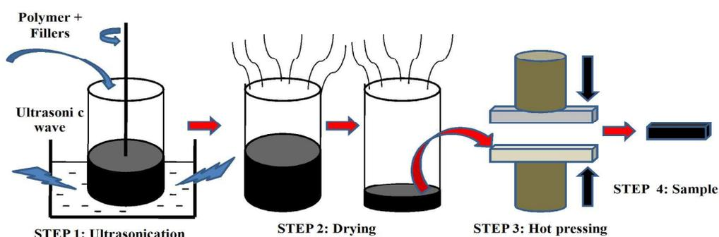
**Scheme 2:** Synthesis and application of thermoelectric polymer nanocomposite
