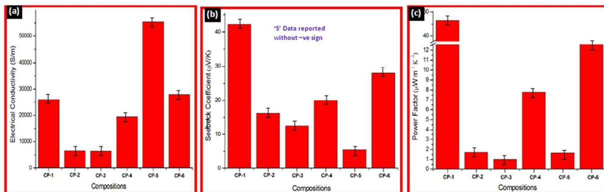
**Fig.6(a)** Electrical conductivity (b) Seebeck coefficient (c) power factor as a function of filler concentration at room temperature (300K) **CP-1:** PVAc (20%), GTNC(80%), **CP-2:** PVAc (15%), PEDOT:PSS (5%), GTNC (80%), **CP-3:** PVAc (10%), PEDOT:PSS (10%), GTNC (80%)**CP-4:** PVAc (5%), PEDOT:PSS (15%), GTNC (80%),**CP-5:**PEDOT: PSS (20%), GTNC (80%), **CP-6:** PEDOT sheet.
