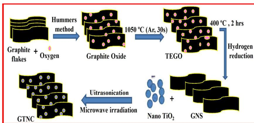
**Scheme 1:** Schematic representation of synthesis of Graphene-Titanium dioxide nano composite (GTNC)
