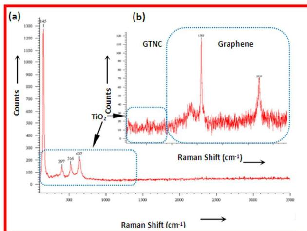
**Fig. 1** (a) represents the Raman traces of nano  $\text{TiO}_2$  and (b) represents GTNC (Gr- $\text{TiO}_2$  composite)
