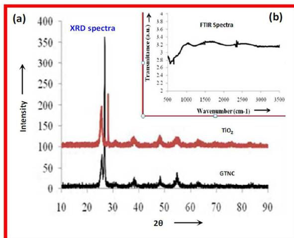
**Fig.2:** XRD profiles of nano TiO<sub>2</sub>, GTNC (Graphene-TiO<sub>2</sub> composite). FTIR traces of graphene are shown in the inset (b).
