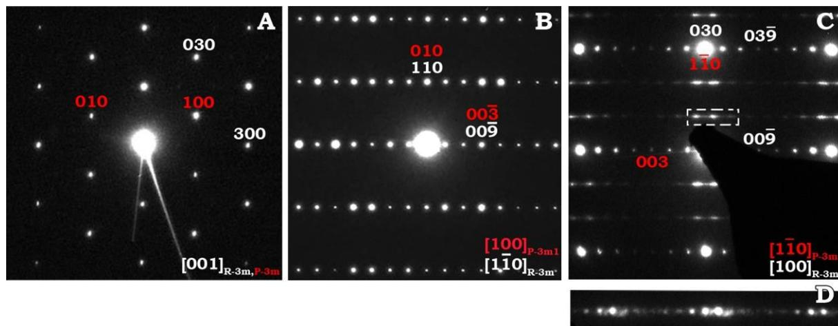
Figure 4. (a-c) Selected area electron diffraction patterns taken along the main zone axis in the crystal. (d) Enlargement from the dashed area in (c). Red and white indices correspond to primitive and rhombohedral centred lattices, respectively.
