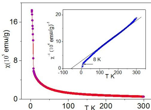
Figure 6. Temperature dependence of the magnetic susceptibility  $\chi$  for  $\text{Ba}_7\text{Li}_{1.75}\text{Mn}_{3.5}\text{O}_{15.75}$  ( $H = 0.3$  kOe). The inset shows the  $\chi^{-1} = f(T)$  dependence.
