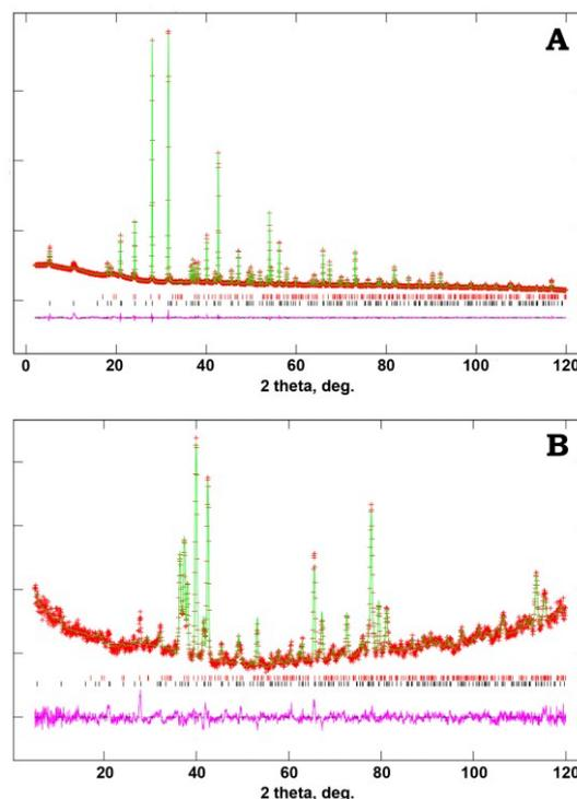
Figure 2. Observed (crosses), calculated (solid line) and difference (bottom line) X-ray (a) and neutron (b) powder diffraction patterns of Ba<sub>7</sub>Li<sub>1.75</sub>Mn<sub>3.5</sub>O<sub>15.75</sub> with BaCO<sub>3</sub> as the impurity phase. Red and black lines show the positions of the peaks of Ba<sub>7</sub>Li<sub>1.75</sub>Mn<sub>3.5</sub>O<sub>15.75</sub> and BaCO<sub>3</sub>, respectively.
