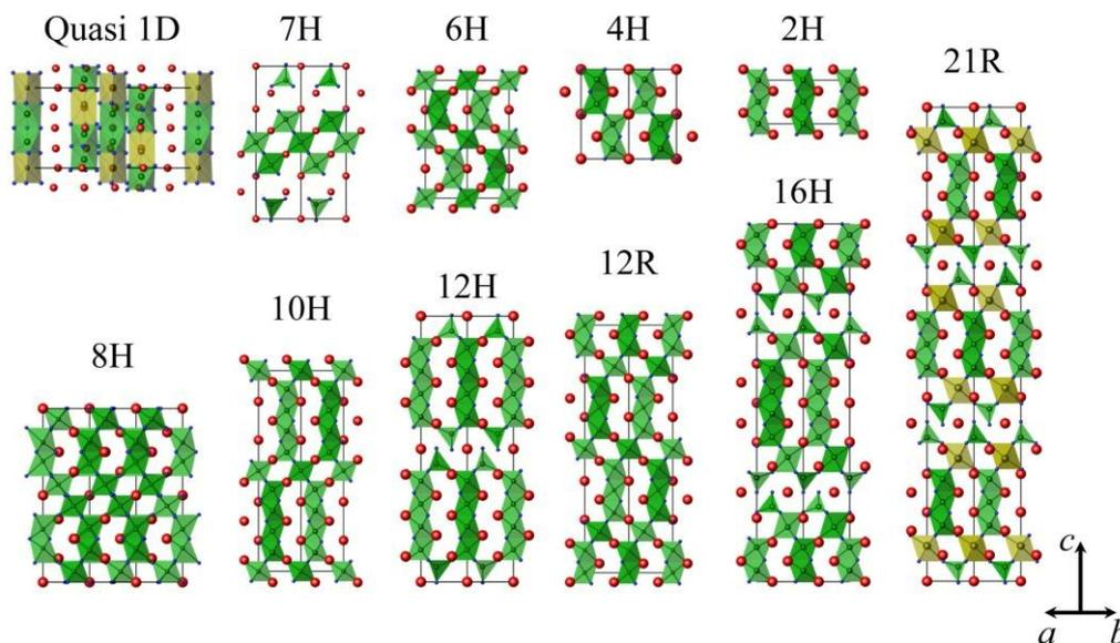
Figure 1. Crystal structures of  $\text{BaMnO}_3$ : different polytypes and quasi-one-dimensional (quasi-1D) compounds  $\text{A}_4\text{A}'\text{Mn}_2\text{O}_9$ . Red and blue spheres indicate A cation and oxygen sites, respectively. Positions indicated by green and yellow polyhedra are preferably occupied by manganese and A' atoms, respectively.
