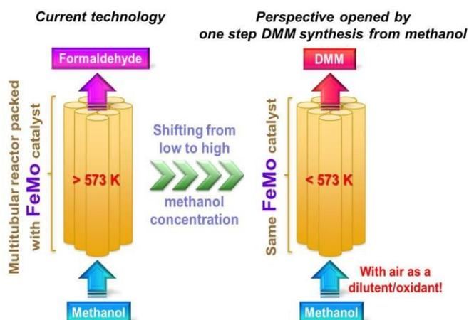
Figure 3 : Concept of transformation of a formaldehyde production plant into a DMM production plant with a FeMo mixed oxides as a versatile catalyst.
