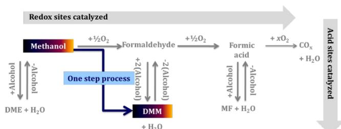
Scheme 1 : Methanol oxidation pathways adapted from <sup>15</sup>.
