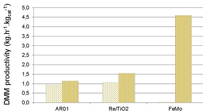
**Figure 2 Evolution of the DMM productivity at 553K for different types of catalysts: Re/TiO<sub>2</sub><sup>105</sup>, FeMo<sup>77</sup> and mixed oxide amorphous material AR01<sup>53</sup> in rich and poor methanol concentration in the feed. Figure adapted from Ref <sup>105</sup>.**
