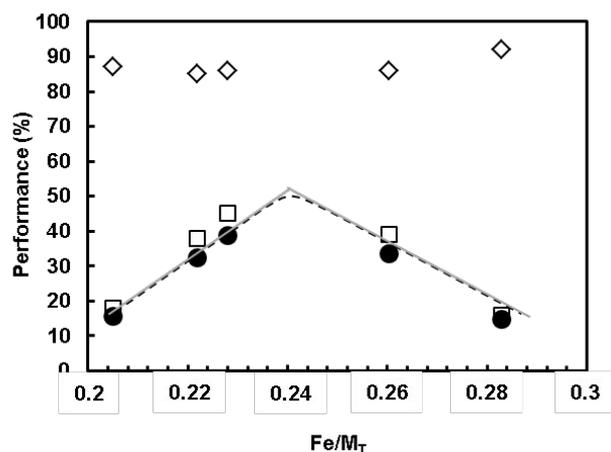
**Figure 1** : Performances at the steady state of FeMo catalysts as a function of the Fe/M<sub>T</sub> molar ratio (with M<sub>T</sub> = Fe + Mo); Methanol conversion (square), DMM selectivity (lozenge), and DMM yield (circle)<sup>12</sup>.
