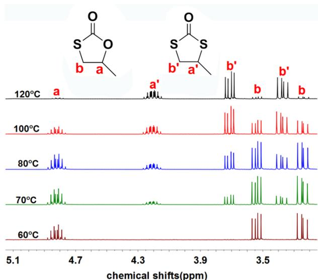
**Figure 1.**  $^1\text{H}$  NMR spectra of the products from PO/COS coupling at different temperatures.  $^1\text{H}$  NMR signals for hydrogens in c and c' positions are further upfield and not shown here, see Figure S28-30.
