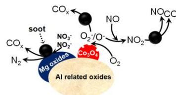
**Scheme 3** Illustration of potential reaction pathways for soot combustion in NO<sub>x</sub>-containing atmosphere over CoMgAlO-array.
