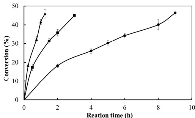
**Fig. 4** Enzymatic resolution of (±)-DmCpCe at 100 mM by *RhEst1* (circle), *RhEst1*<sub>A147V/G254A</sub> (square) or *RhEst1*<sub>A147I/V148F/G254A</sub> (triangle) at a catalyst loading of 5 g L<sup>-1</sup> of lyophilized cell-free extract. The reaction was conducted in Tris-HCl buffer (pH 8.0, 200 mM) at 25°C.
