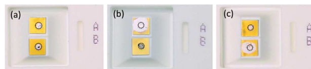
Fig. 4 Subtyping influenza viruses with photopolymerization-based signal amplification. (a) No virus detected so polymer is only observed within the positive control spots. (b) Influenza A detected. (c) Influenza B detected. Reprinted with permission from Sikes et al., Lab on a Chip , 2009, 9, 633-656. Copyright © 2009, The Royal Society of Chemistry. 13
