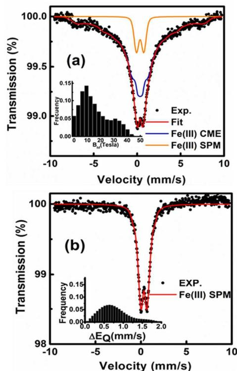
Figure 4 Mössbauer spectra for the iron oxide nanoparticles at 300 K prepared in (a) argon atmosphere, and (b) Vacuum conditions.
