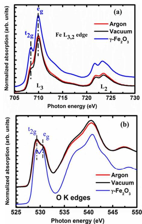
Figure 3 (a) Fe L<sub>3,2</sub> edges and (b) O K edges XANES recorded in TEY mode for iron oxide nanoparticles prepared in argon atmosphere, and vacuum conditions along with reference compound  $\gamma$ -Fe<sub>2</sub>O<sub>3</sub>.
