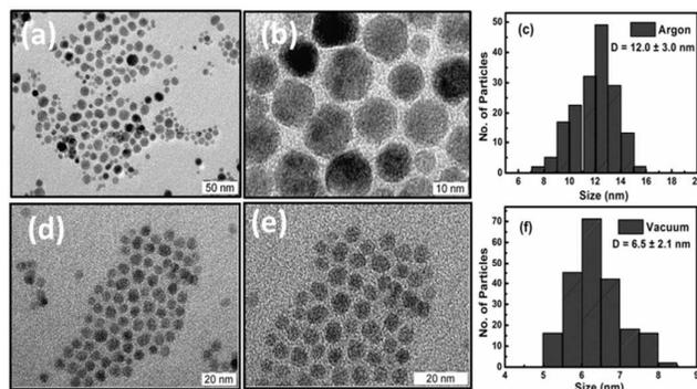
Figure 2 TEM images for iron oxide samples prepared in Argon atmosphere (a-c) and vacuum (d-f) along with their particle size distribution histograms.
