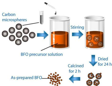
Fig. 1. Schematics for the synthesis of the samples via a carbon microsphere-assisted sol-gel method
