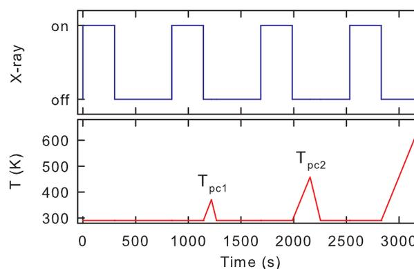
**Fig. 1** Scheme of the irradiation and heating profiles used for YAG:Ce,Lu and LSO:Ce samples
