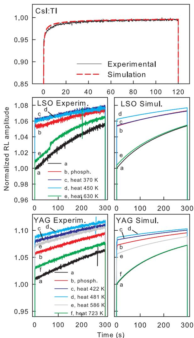
**Fig. 3** Experimental and simulated bright burn curves of CsI:Tl, LSO:Ce, and YAG:Ce,Lu. The measurements have been performed at 290 K in the case of LSO:Ce and YAG:Ce,Lu samples, and at 283 K for CsI:Tl one. The curves have been normalized to the maximum of the RL signal in the case of CsI:Tl, and to the first non-zero point of the first measurement in the case of the two oxides.
