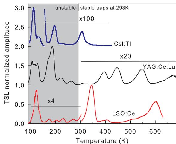
**Fig. 2** Normalized TSL glow curves obtained after irradiation at 85 K of the three investigated samples. The heating rate of the presented curve is 0.1 K/s for LSO:Ce and YAG:Ce,Lu, and 0.5 K/s for CsI:Tl. The curves have been shifted along the ordinate axis for clarity
