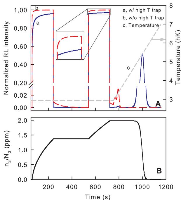
**Fig. 4** Simulation of an irradiation-phosphorescence-irradiation-thermoluminescence measurement scheme: A) comparison between a two trap model and a three trap one, starting from the results obtained on CsI:Tl presented in Fig. 3. The added third trap has  $E = 1.74$  eV and concentration equal to  $10^{19}$   $\text{cm}^{-3}$ . B) Calculated occupation ratio of the third trap as a function of time
