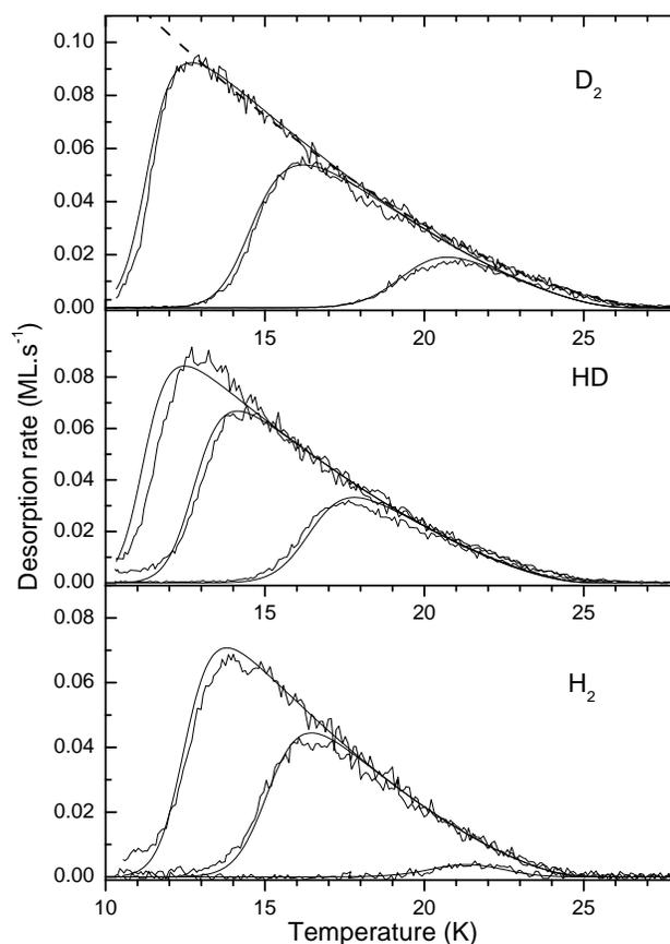
**Fig. 1** Set of three TPD experiment for H<sub>2</sub>, HD and D<sub>2</sub>. Exposure doses in ML : 0.7, 1.4 and 2.6 for H<sub>2</sub>; 1.0, 2.4 and 3.3 for HD; 0.5, 2.0 and 4.0 for D<sub>2</sub>. Smooth lines are model adjustment (see section 3). Dashed line on top panel shows a  $(T_0 - T)^{1.6}$  law for the trailing edge
