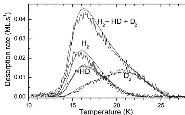
**Fig. 3** TPD experiment for a mixed sub-monolayer adsorption of isotopologues: H<sub>2</sub> 1.3 ML, HD 1.0 ML and D<sub>2</sub> 0.7 ML. An artificial TPD for molecular hydrogen desorption regardless its isotope nature has been plotted summing up the three curves. Smooth lines: Results of simulation, see section (3).
