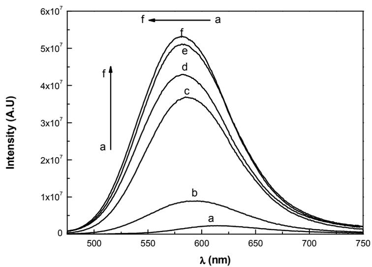
**Figure 1.** Emission spectra of HC in AOT-BHD unilamellar vesicles varying [AOT-BHD]. [AOT-BHD]: a) 0 mg/mL, b) 0.1 mg/mL, c) 0.5 mg/mL, d) 1 mg/mL, e) 3 mg/mL, f) 5 mg/mL,  $\lambda_{\text{exc}} = 450$  nm. [HC] =  $1 \times 10^{-5}$  M.
