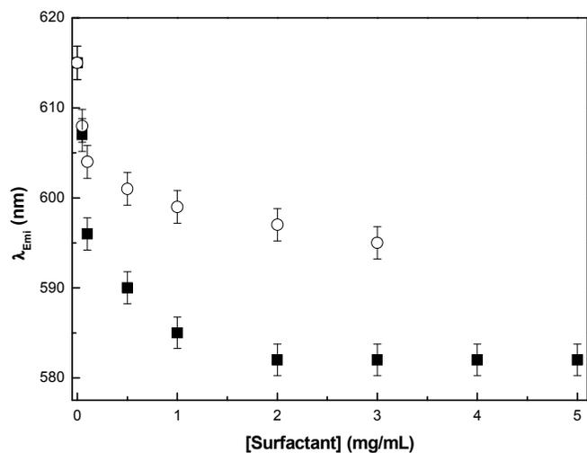
**Figure 2.** Variation of HC emission wavelength maxima ( $\lambda_{em}$ ) as a function of [surfactant] in AOT-BHD (■) and DOPC (○) vesicles.  $\lambda_{exc} = 450$  nm.  $[HC] = 1 \times 10^{-5}$  M. DOPC values taken from reference 58.
