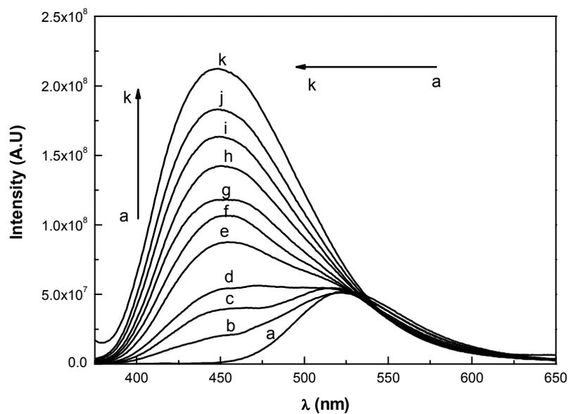
**Figure 5.** Emission spectra of PRODAN in AOT-BHD unilamellar vesicles varying [AOT-BHD]. [AOT-BHD]: a) 0 mg/mL, b) 0.05 mg/mL, c) 0.1 mg/mL, d) 0.25 mg/mL, e) 0.5 mg/mL, f) 0.75 mg/mL, g) 1 mg/mL, h) 1.5 mg/mL, i) 2 mg/mL, j) 3 mg/mL, k) 5 mg/mL.  $\lambda_{\text{exc}} = 350 \text{ nm}$ . [PRODAN] =  $5 \times 10^{-6} \text{ M}$ .
