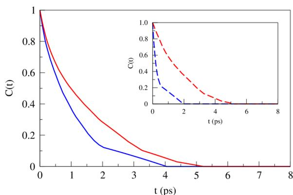
**Fig. 4** Continuous population autocorrelation functions of water binding on iron sites of FeS<sub>2</sub> (100) surface. Blue: normal surface; red: defective surface. Inset: The same functions calculated for different sites on the defective surface. Blue: 5-coordinated surface iron atoms; red: 4-coordinated (defective) surface iron atoms.
