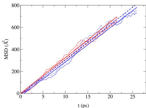
**Fig. 2** Mean square displacements as a function of time. Red: on normal surface; blue: on defective surface. Solid line: total displacement; dashed line: displacement parallel to the  $xy$  directions. Fitted straight lines are also shown.
