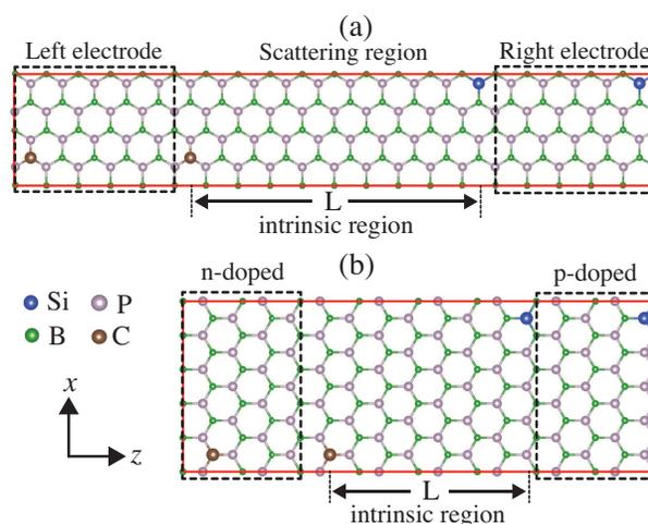
**Fig. 4** The device models: for (a) zigzag and (b) armchair  $p$ - $n$  junction.
