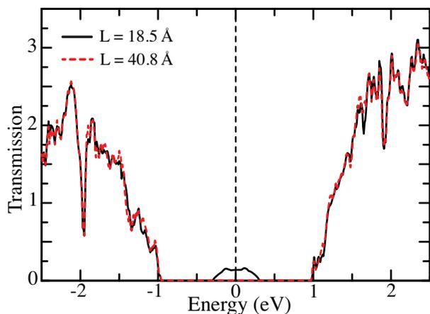
**Fig. 7** Zero bias transmission spectrum of armchair  $p$ - $n$  junction for two different intrinsic region length ( $L$ ).
