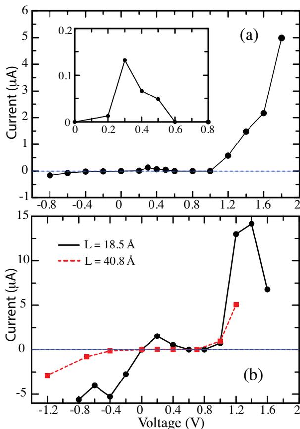
**Fig. 5** The calculated current-voltage (I-V) curves for (a) zigzag and (b) armchair terminated  $p$ - $n$  junction. Inset in (a) shows I-V for  $V=0-0.8$  V. In (b) I-V curves for armchair terminated  $p$ - $n$  junction with two different intrinsic region sizes are shown.
