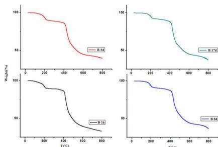
**Figure 2a.** Thermogravimetric profiles of benzene/compound **1** after stored for different time.
