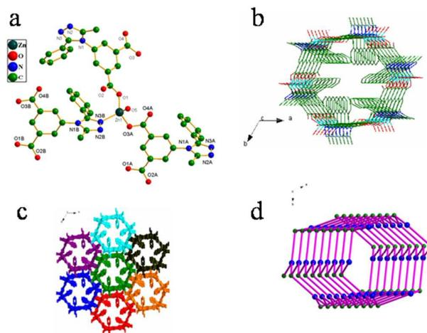
**Figure 1.** (a) Coordination environment of the Zn<sup>II</sup> ion (All hydrogen atoms and solvent molecules are omitted for clarity). (b) Structure of 1D tube for **1** (All solvent molecules are omitted for clarity). (c) 3D structure of **1** running along the *ab*-plane. (d) Topology of **1** along the *ab*-plane.
