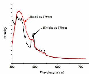
**Figure 3.** Solid state emission spectra for compound **1** and the ligand H<sub>2</sub>L at room temperature.
