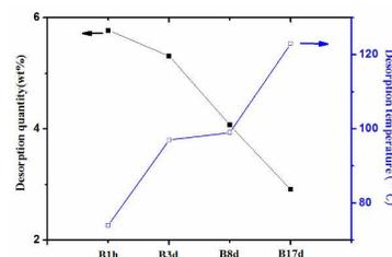
**Figure 2b.** Desorption quantities and temperatures of benzene/compound **1** after stored for different time.
