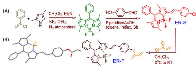
Scheme 1: (A) Methodologies adopted for the synthesis of **ER-F**; (B) Single-crystal X-ray structure of probe **ER-F** [Hydrogen atoms are omitted for clarity].<sup>†</sup>
