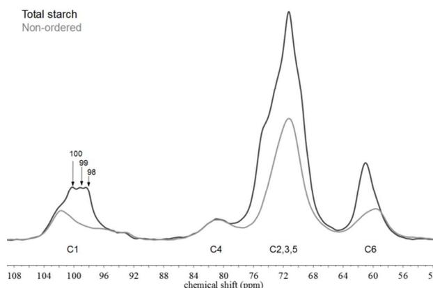
**Figure 1.** Exemplar  $^{13}\text{C}$  CP/MAS NMR spectra for semi-crystalline A-type starch (black) and non-ordered (amorphous) starch (grey) with the assignments of each of the peaks indicated.
