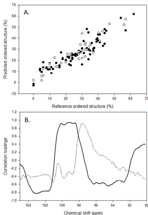
**Figure 3.** PLS model constructed using the C1 region of the  $^{13}\text{C}$  CP/MAS NMR spectra for starch. a. Reference vs. predicted ordered helical structure for calibration samples (filled circles) and validation samples (open circles). b. Model correlation loadings for principle component 1 (solid line) and principle component 2 (broken line)
