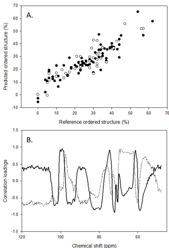
**Figure 2.** PLS model constructed using the full  $^{13}\text{C}$  CP/MAS NMR spectra for starch. a. Reference vs. predicted ordered helical structure for calibration samples (filled circles) and validation samples (open circles). b. Model correlation loadings for principle component 1 (solid line) and principle component 2 (broken line)
