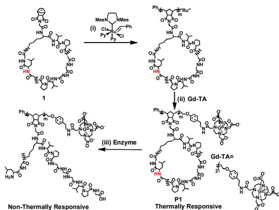
**Fig. 1.** Synthetic scheme of homopolymer **P1** using ROMP initiator (IMesH<sub>2</sub>)(C<sub>5</sub>H<sub>5</sub>N)<sub>2</sub>(Cl)<sub>2</sub>Ru=CHPh (“Ru”) and Gd-containing termination agent (Gd-TA). For **P1**, *m* = 5. The structure post-enzyme treatment is drawn to represent the ideal result of 100% peptide cleavage. Enzyme cleavage site is shown in red color.
