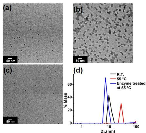
**P2 micelles:** at room temperature (black curve), at 55 °C for 6 h (red curve), with enzyme at 55 °C for 6 h (blue curve).
