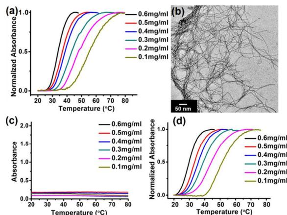
**Fig. 3** (a) LCST behavior of **P1** measured by UV-Vis spectroscopy at 550 nm; (b) TEM image of cylindrical structure formed by **P1** (0.6mg/ml) at 40°C. (c) LCST behavior of **P1** treated with thermolysin at 55 °C for 1 h. (d) LCST behavior of **P1** treated with denatured thermolysin at 55 °C for 1 h.
