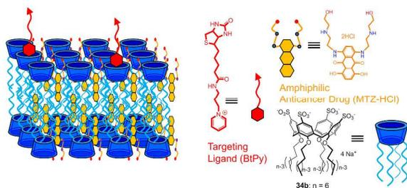
**Figure 14:** Co-assembly of tetrahexyloxy-p-sulfonatocalix[4]arene **34b** and cationic amphiphilic anticancer drugs (Mitoxantrone hydrochloride MTZ-HCl) into a double layer of micelles. Noncovalent surface modification with a pyridinium functionalized biotin allows targeted drug-delivery.
