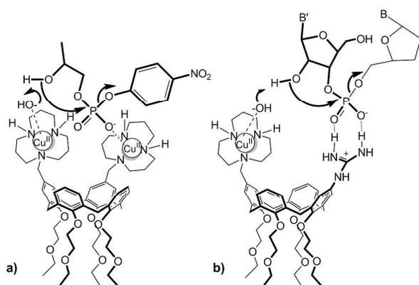
**Figure 12:** Proposed mode of a) HPNP transesterification, catalyzed by **22-Cu<sub>2</sub>**; b) RNA-dinucleotide transesterification, catalyzed by **25-Cu**.
