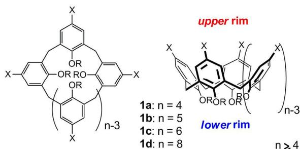
**Figure 1:** The planar representation (left) and a three-dimensional sketch (right) of the calix[n]arenes **1** ( $n \geq 4$ ) with the indications of the two rims.
