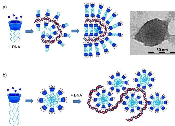
**Figure 11:** Different proposed mechanism of DNA compaction for calixarenes **17a** and **18**. (a) DNA binding followed by aggregation of the facial calixarene amphiphile **17a**; on the right, the snake-like ultra-thin structure evidenced by a TEM image is reported. (b) The self-aggregation of the amphiphile **18** followed by DNA binding (hierarchical self-assembly).
