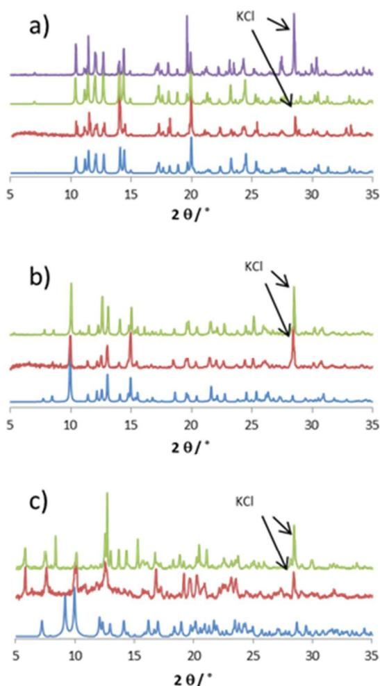
**Figure 2.** PXRD: a) From bottom to top calculated for **5a**, measured for **5a** (reaction product), calculated for **6a** and measured for **6a** (reaction product). b) From bottom to top calculated for **5b**, measured for **5b** (reaction product) and **6b** (reaction product); c) From bottom to top calculated for **5c**, measured for **5c** (reaction product) and **6c** (reaction product).
