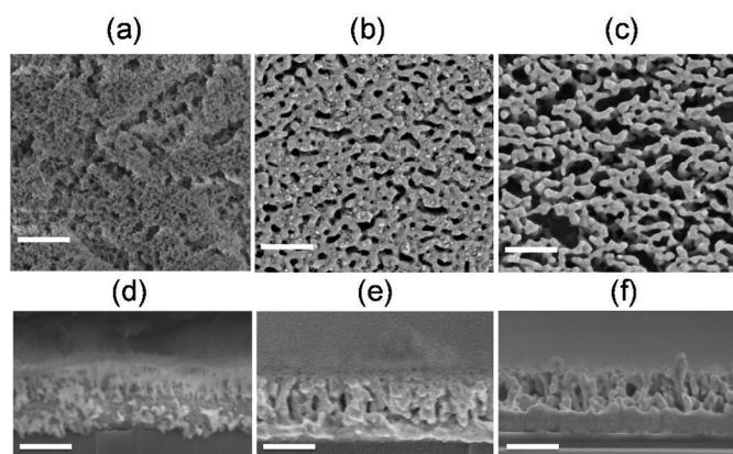
**Fig. 1** Representative FE-SEM images of bare nanoporous Au films on a Si wafer. (a, b, c) Show top views and (d, e, f) show cross sectional views of np-Au-1, np-Au-2, and np-Au-3, respectively, with different levels of porosity based on the amount of de-alloyed Si in each catalyst. The resulting RFs of np-Au-1, np-Au-2, and np-Au-3 are 2.48, 31.1, and 22.89, respectively. The thickness of the nanoporous Au is ~150–200 nm (scale bar refers to 200 nm).
