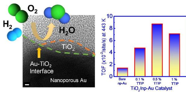
Catalytic activity of nanoporous Au prepared from a Au-Si alloy is enhanced by engineering Au-TiO<sub>2</sub> interfaces under H<sub>2</sub> oxidation
