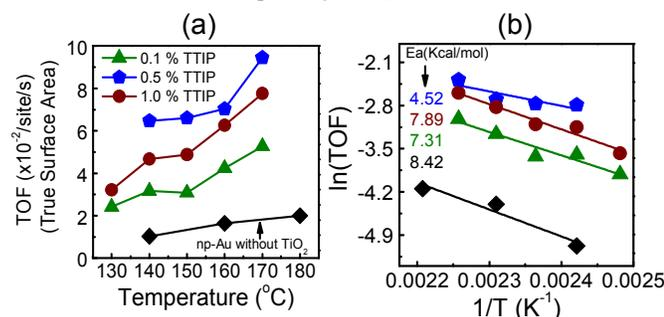
**Fig. 3** Catalytic activity of H<sub>2</sub> oxidation on TiO<sub>2</sub>/np-Au catalysts: (a) turnover frequency as a function of temperature and (b) Arrhenius plots and activation energies (E<sub>a</sub>) in kcal/mol. Compared to bare nanoporous Au, the TOF is enhanced after TiO<sub>2</sub> deposition via TTIP impregnation.
