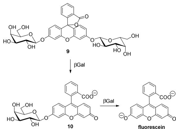
**Fig. 4** Sequential FDG hydrolysis to yield fluorescein.
