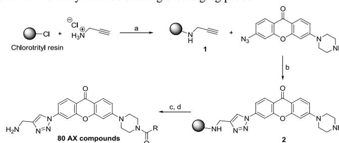
**Scheme 1** Synthesis of AX library. Reagents and Conditions: (a) DIEA, DMF/DCM, r.t, 12 h; (b) CuI, Ascorbic acid, DMF/Piperidine (4:1), r.t, 24 h; (c) DIEA, RCOCl DCM, r.t, 4 h; (d) 2% TFA in DCM, r.t, 15 min.
