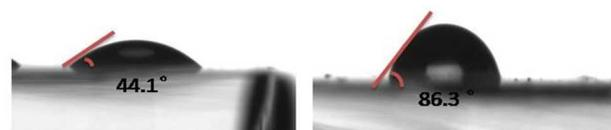
**Figure 5.** The static contact angle of perovskite film (left) and C<sub>12</sub>-silane/perovskite (right) film with the de-ionized water.
