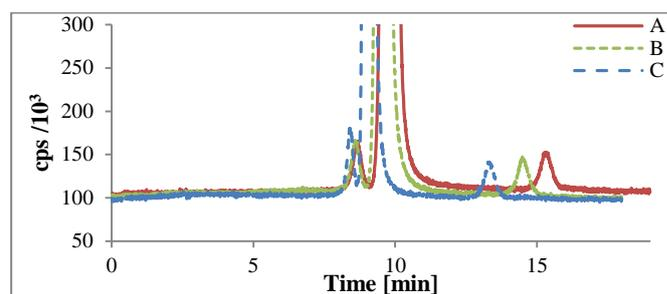
**Fig. 3** IC-ICPMS gradient time optimisation, detected at m/z 35. **A:** 10–80 mM KOH in 0–5 min. **B:** 10–80 mM KOH in 0–3 min. **C:** 10–80 mM KOH in 0.00–0.01 min.
