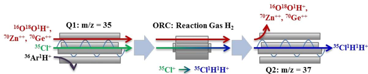
**Fig. 5** Chlorine determination by ICPQQMS in MS/MS mode with  $\text{H}_2$  as reaction gas.
