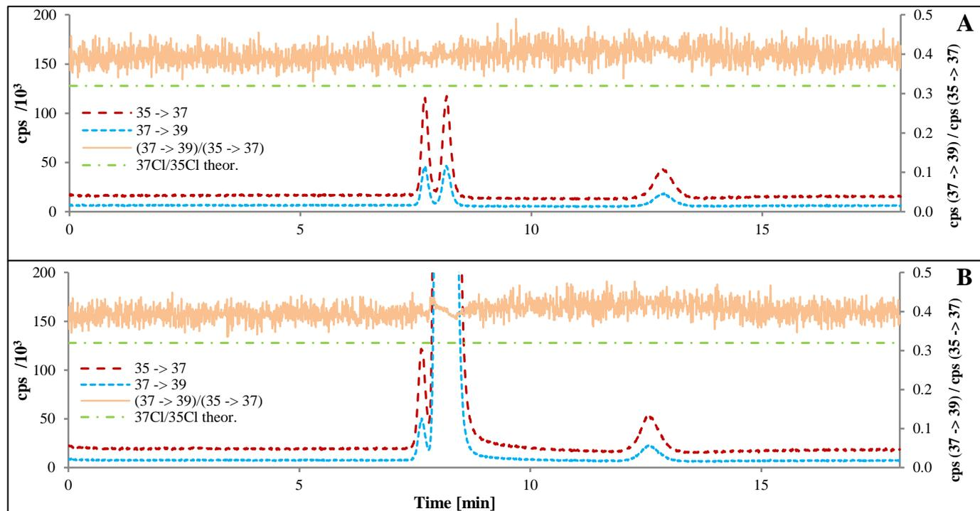
**Fig. 6** Chlorine speciation analysis by IC-ICPQQMS. **A:** Standard solution (5.0 mg Cl L<sup>-1</sup>) **B:** Horse plasma spiked with chlorite and chlorate (5.0 mg Cl L<sup>-1</sup>). Recovery of chlorite 93 % and of chlorate 104 %.
