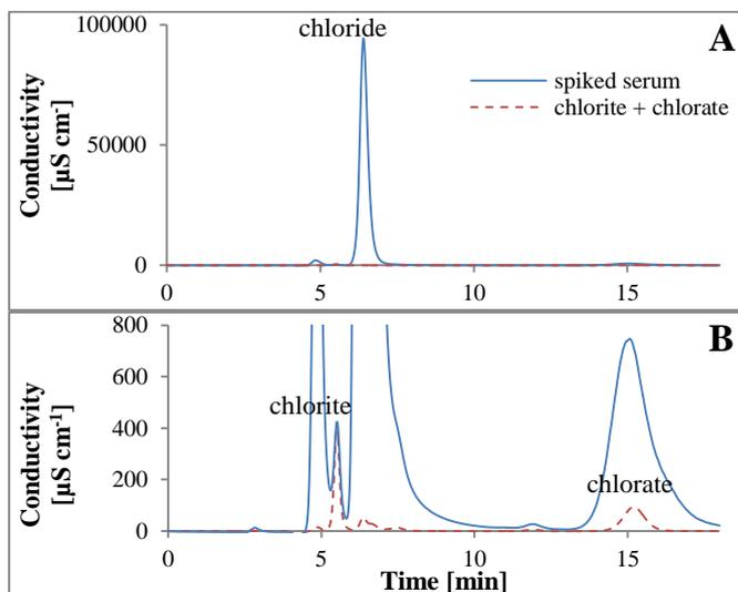
**Fig. 1:** IC chromatograms (30 mM KOH isocratic with suppressed conductivity detection) of a reference serum (1+9) spiked with 1.0 mg  $\text{Cl L}^{-1}$  chlorite and chlorate and a standard of 1.0 mg  $\text{Cl L}^{-1}$  chlorite and chlorate. **A:** Full-size serum chromatogram. **B:** Zoom in on the baseline.
