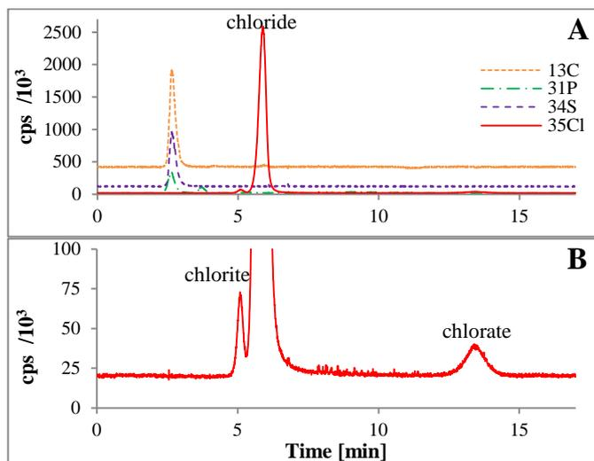
**Fig. 2** IC-ICPMS chromatograms (40 mM KOH isocratic) of a sample containing serum (1+9) spiked with 5.0 mg L<sup>-1</sup> chlorite and chlorate. Shown are the mass traces of carbon <sup>13</sup>C, phosphorous <sup>31</sup>P, sulfur <sup>34</sup>S (representing parts of the matrix) and chlorine <sup>35</sup>Cl. **A:** All chromatograms. **B:** Zoom in on the chlorine baseline.
