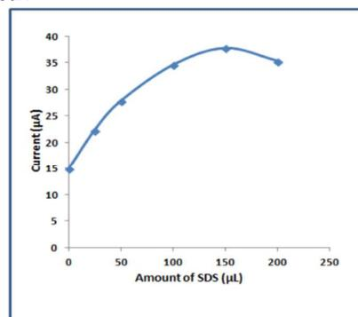
**Fig.2** The effects of different amount of SDS on the sensor response for 5.0x10<sup>-5</sup> M DA. Conditions: in 6.7x10<sup>-2</sup> M phosphate buffer solution (PBS) (pH 7.0), working potential: -0.5 V - +0.7 V and scan rate 100 mVs<sup>-1</sup>.
