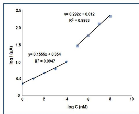
**Fig.6** Calibration graph for DA concentrations between  $1.0 \times 10^{-9}$  M –  $1.0 \times 10^{-5}$  M and  $2.0 \times 10^{-5}$  M –  $1.0 \times 10^{-1}$  M. Centrifugation speed 5000 rpm, centrifugation time 5 min.
