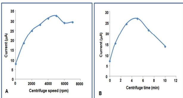
**Fig.3** The effects of centrifugation parameters on the sensor response, **A)** centrifuge speed, **B)** centrifuge time for  $5.0 \times 10^{-5}$  M DA. Conditions: in  $6.7 \times 10^{-2}$  M PBS (pH 7.0) in presence of  $6.7 \times 10^{-5}$  M  $150 \mu\text{L}$  SDS, working potential:  $-0.5$  V  $+0.7$  V and scan rate  $100$  mVs $^{-1}$ .
