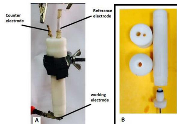
**Scheme 1.** Illustration of centri-voltammetric cell, A) on the stand, B) the parts of centri-voltammetric cell.
