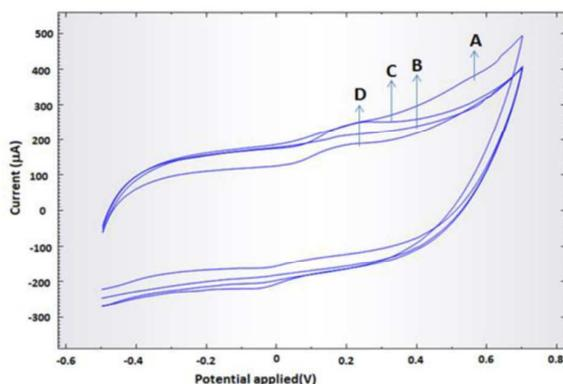
**Fig.5** CV voltammograms show the effects of SDS and centri-voltammetry for electrochemical detection of  $5.0 \times 10^{-5}$  M DA. **A)** without SDS and centrifuge, **B)** with SDS and without centrifuge, **C)** with SDS and centrifuge and **D)** without SDS and with centrifuge.
