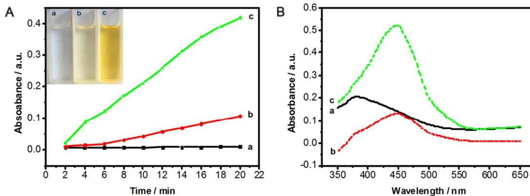
Fig. 3 (A) Time- and (B) wavelength-dependent absorbance changes of OPD at 450 nm in different reaction systems: (a) OPD + CuS nanorods, (b) OPD + H<sub>2</sub>O<sub>2</sub>, and (c) OPD + CuS nanorods + H<sub>2</sub>O<sub>2</sub> in a pH 4.0 HAc-NaAc buffer (0.1 M) at room temperature. Inset shows the color change of different samples.
