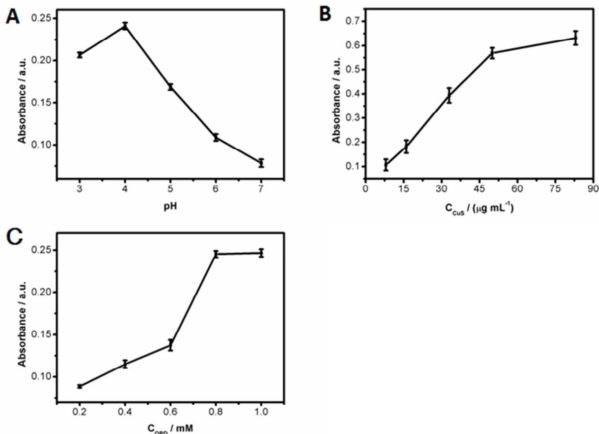
Fig. 6 Effects of (A) pH, (B) concentration of CuS nanorods, (C) Concentration of OPD on the absorbance in the color reaction with the  $\text{H}_2\text{O}_2$  concentration of 0.1 mM.
