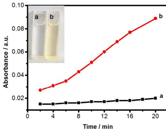
Fig. 4 Time-dependent absorbance evolution of OPD oxidation system at 450 nm in the presence of CuS nanorods (a) and leaching solution (b). Inset shows the color change of different samples.
