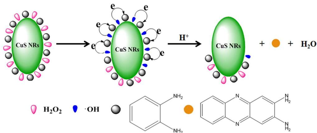
Scheme 2. The possible catalytic mechanism of CuS nanorods.
