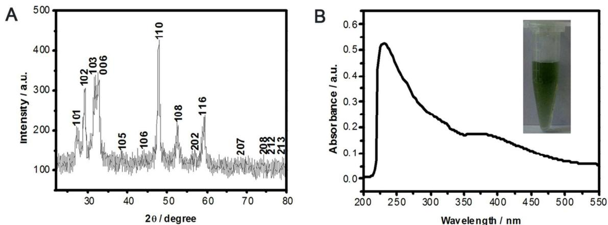
Fig. 2 (A) XRD and (B) UV-vis spectra of of as-synthesized CuS nanorods. Inset of B is the photograph of CuS nanorods dispersed in water.
