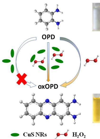
Scheme 1 Schematic representation of the colorimetric detection of hydrogen peroxide based copper sulfide nanorods as peroxidase mimetics.
