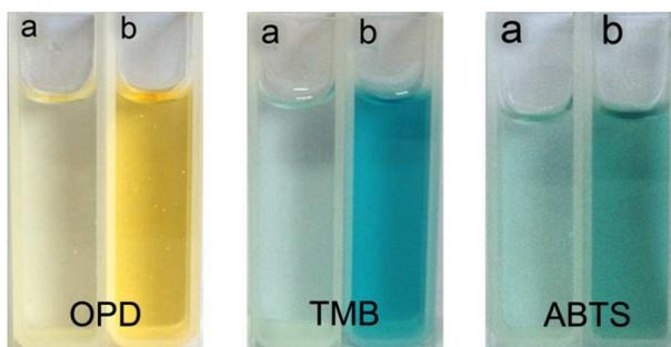
Fig. 5 Images of oxidation color reaction of OPD, TMB, and ABTS by H<sub>2</sub>O<sub>2</sub> before and after by the catalysis of CuS nanorods, respectively.
