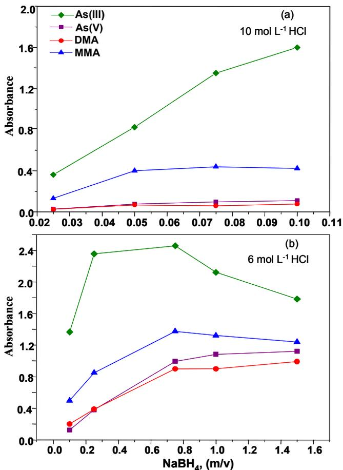
**Fig. 4.** Influence of  $\text{NaBH}_4$  concentration on the absorbance of As species ( $10 \mu\text{g L}^{-1}$  each); DMA: dimethylarsinic acid; MMA: monomethylarsonic acid.
