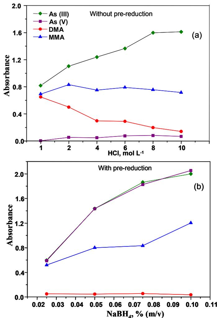
**Fig. 3** Influence of HCl and NaBH<sub>4</sub> concentrations on the absorbance of As species (10  $\mu\text{g L}^{-1}$  each); DMA: dimethylarsinic acid; MMA: monomethylarsonic acid. The NaBH<sub>4</sub> and HCl concentrations were 0.1% (a) and 10 mol L<sup>-1</sup> (b), respectively. The absorbances in (b) correspond to As species submitted to pre-reduction using KI (5% m/v) + ascorbic acid (1% m/v).
