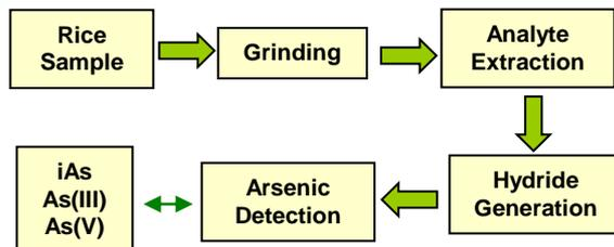
Inorganic arsenic (iAs) is very toxic. iAs in rice was determined using selective hydride generation conditions and atomic absorption spectrometry.
