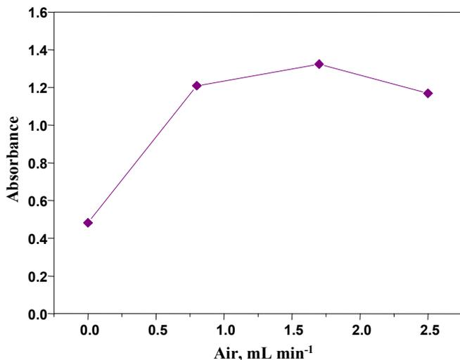
**Fig. 2** Influence of air introduced into the gas-liquid separator on the absorbance of As (III) (10  $\mu\text{g L}^{-1}$  in 1 mol L<sup>-1</sup> HCl); NaBH<sub>4</sub> concentration: 0.5% m/v. See Fig. 1 for additional information.
