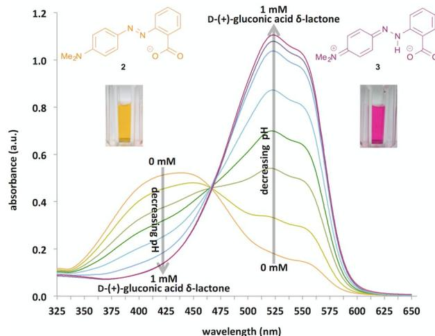
Fig. 6 Stacked UV/vis spectra (25 °C) of methyl red solutions (0.05 mM **2** in water) that were exposed to different concentrations of D-(+)-gluconic acid  $\delta$ -lactone (0–1 mM).
