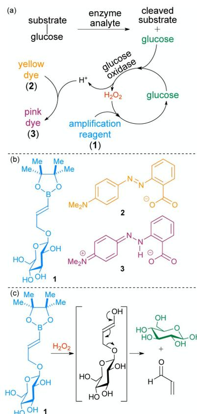
Fig. 2 (a) The amplification strategy employed in this work; (b) structures of specific reagents used in the assay; and (c) partial mechanism of response of the signal amplification reagent. The signal amplification reagent, **1**, is blue, the propagating signal,  $\text{H}_2\text{O}_2$ , is red, and the generated product, glucose, is green, which are colors that match the coding in Fig. 1.
