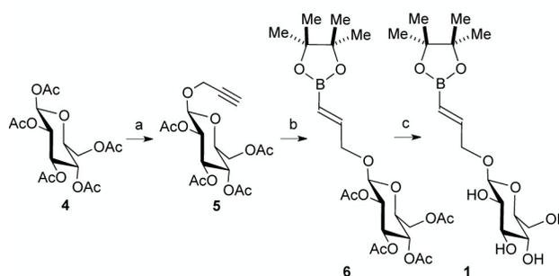
Fig. 4 Synthesis of amplification reagent **1**. Conditions: a, propargyl alcohol,  $\text{BF}_3 \cdot \text{Et}_2\text{O}$  (89%); b, pinacolborane, 100 °C (37%); c, (i) NaOMe, MeOH,  $\text{CH}_2\text{Cl}_2$ ; (ii) Dowex  $\text{H}^+$  (80%).
