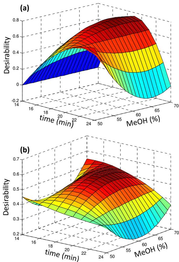
Fig. 2. Optimization of the separation by experimental design. (a) Study with standards using a desirability function  $D = (d_{R_{s,s/e}} \times d_{R_{s,f/s}} \times d_{t_R})^{1/3}$  that considers resolution of syringic acid and epicatechin, ferulic and salicylic acids and analysis time. (b) Study on beer using a desirability function  $D = (d_{\text{peak}} \times d_{t_R})^{1/2}$  that considers number of resolved peaks and analysis time.
