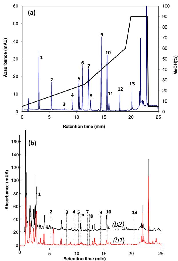
Fig. 3. Chromatograms obtained with the optimized separation. (a) Standards at  $5 \text{ mg L}^{-1}$ ; the gradient profile is overlapped. Peak assignment: 1: gallic acid, 2: protocatechuic acid, 3: 2,5-dihydroxybenzoic acid, 4: catechin, 5: vanillic acid, 6: caffeic acid, 7: syringic acid, 8: epicatechin, 9: *p*-coumaric acid, 10: ferulic acid, 11: salicylic acid, 12: rutin, 13: quercetin. (b) Beer samples: b1, lager; b2, ale.
