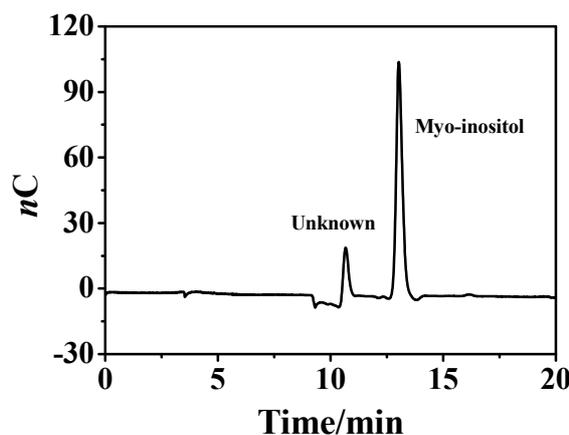
Fig. 9 Chromatogram of myo-inositol in infant formula sample after matrix elimination with column-switching.
