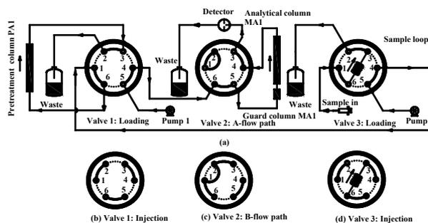
Fig. 2 Instrument configuration for the analysis of myo-inositol in milk powder sample: (a) filling the sample loop; (b-d) the positions of valves 1, 2 and 3; the flow path was shown as the bold line.
