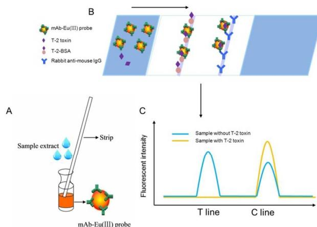
Fig. 2 Schematic sketch of the LF-TRFIA method
