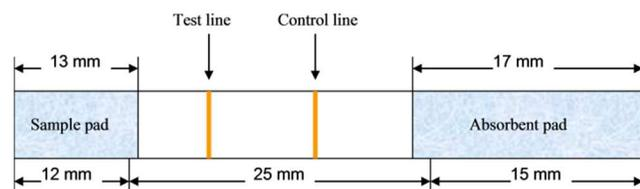
Fig. 1 Constructional detail of the immunochromatographic assay strip
