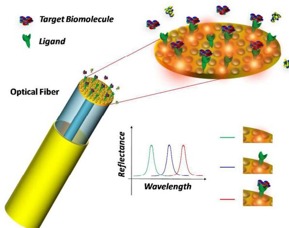
**Fig. 2** Schematic of the Lab-On-Fiber biosensing principle. A metallic nanostructure supporting a resonant plasmonic mode is integrated on the optical fiber tip. When a molecular binding event occurs at the sensor surface, the reflectance peak associated to the plasmonic mode shifts towards longer wavelengths.
