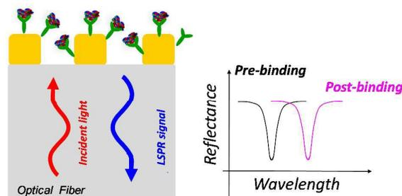
**Fig. 3** Operating principle schematic of the LSPR-based optical fiber probe. A red shift of LSPR peak is observed in the reflection spectrum when the analyte interacts with the ligand on the surface of a metal nanostructure.
