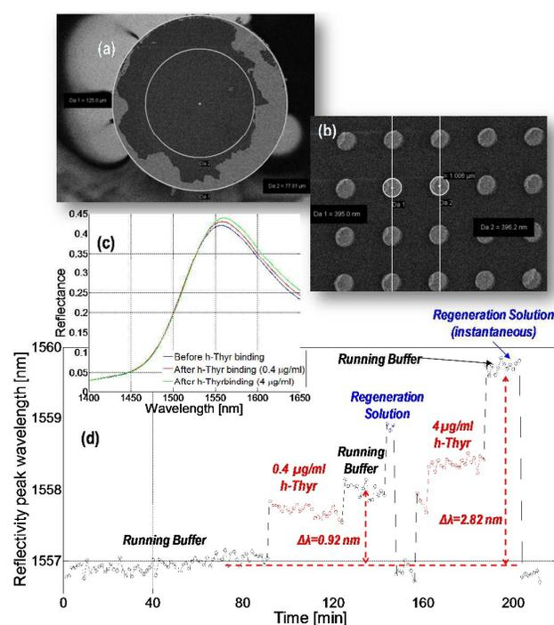
**Fig. 4** (a) SEM image (top view) of the optical fiber probe; (b) zoomed-in image of (a); (c) Experimental reflection spectrum of the fabricated device before and after the h-Thyr binding ( $0.4 \mu\text{g}/\text{mL}$  and  $4 \mu\text{g}/\text{mL}$ ) in PBS; (d) Sensorgram obtained for the detection of  $0.4 \mu\text{g}/\text{mL}$  and  $4 \mu\text{g}/\text{mL}$  of h-Thyr. The baseline regeneration step is also shown.
