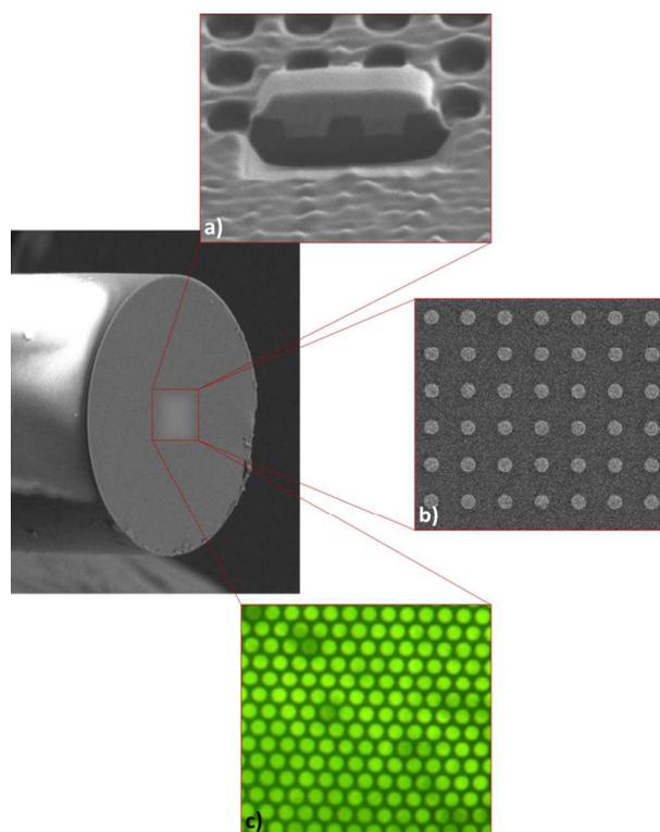
**Fig. 1** SEM images of nanopatterning realized onto optical fiber tip via top-down approach (a, b) and a fluorescence microscopy image of a nanostructure obtained through the bottom up approach (c).
