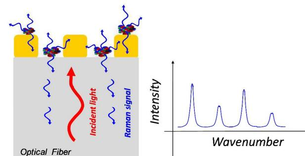
**Fig. 5** Operating principle schematic of the SERS-based optical fiber probe. LSPR excitation supported by the metallic nanostructure transfers energy to the target molecule immobilized on the surface, allowing the enhancing of the Raman signal and vibrational modes to be detected.
