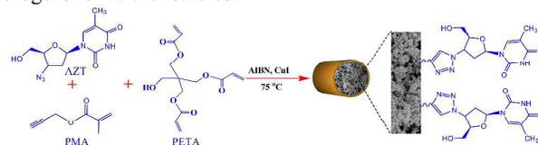
Fig.1. Scheme for one-pot synthesis of the poly (AZT-co-PMA-co-PETA) monolithic column based on *in situ* free radical polymerization combined with CuAAC click reaction.
