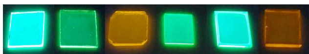
Fig. 3. The photo picture of Borebt1–6 (from left to right) in drop-cast film ( \lambda_{\text{ex}} = 365 nm using a UV lamp).
