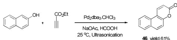
**Scheme 12** Synthesis of a benzo[*f*]coumarin through a palladium catalyzed cyclization.
