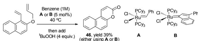
**Scheme 23** Synthesis of benzo[*f*]coumarin through ring closing olefin metathesis (RCM).
