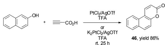
**Scheme 17** Synthesis of a benzocoumarin through Pt-catalyzed aryl C-H functionalization.
