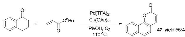
**Scheme 14** Metal catalyzed route to benzo[*h*]coumarin from 3,4-dihydronaphthalen-1(*2H*)-one.
