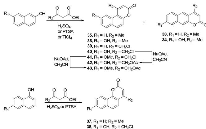
**Scheme 8** Synthesis of benzocoumarins through the Pechmann reaction.
