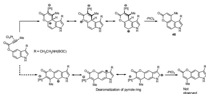
**Scheme 16** Mechanism of metal catalyzed aryl C-H functionalization.
