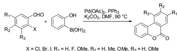
Scheme 32 Synthesis of benzo[*c*]coumarins from *o*-halogenobenzaldehydes and *o*-hydroxybenzeneboronic acids.
