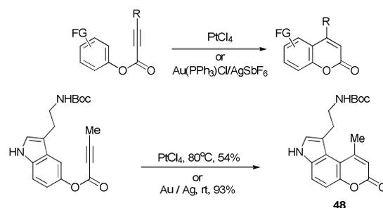
**Scheme 15** Nobel metal catalyzed synthesis of benzocoumarin and pyrrolocoumarin derivatives.
