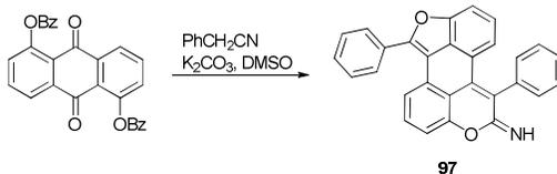
**Scheme 53** The synthesis of  $\pi$ -expanded iminocoumarin.
