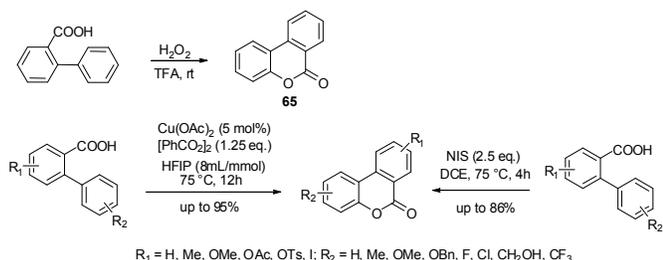
**Scheme 34** Oxidative radical cyclization of biphenyl-2-carboxylic acids.
