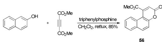
**Scheme 22** Synthesis of benzocoumarin through the Wittig condensation.
