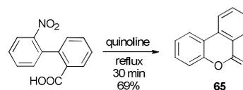
Scheme 33 Nucleophilic substitution of nitro group in 2'-nitrobiphenyl-2-carboxylic acids.
