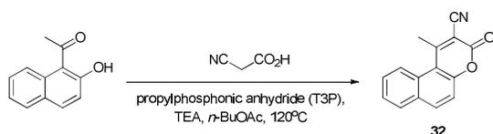
**Scheme 7** Synthesis of benzocoumarin through the Perkin condensation.
