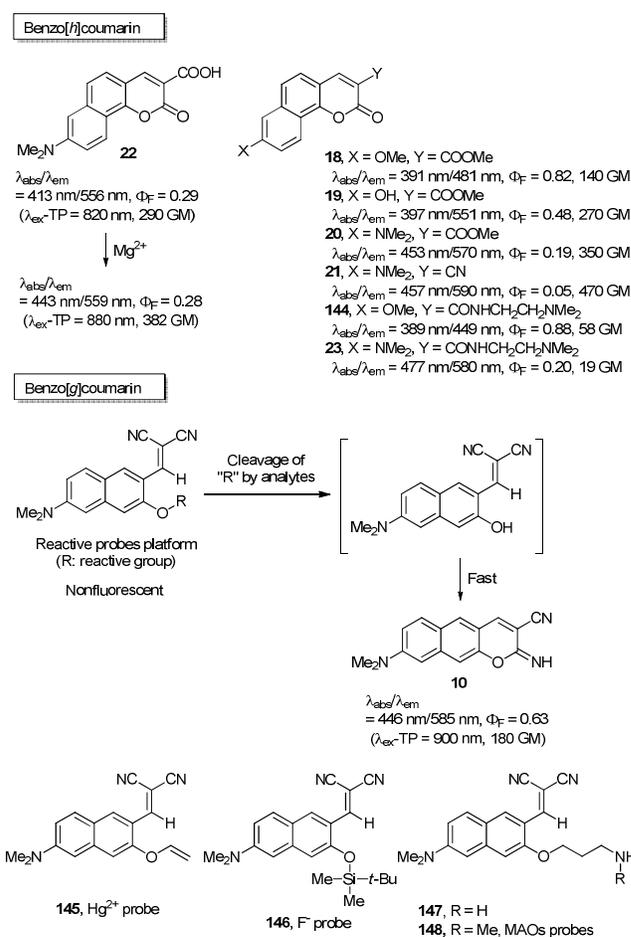
**Scheme 55** Benzo[*h*]coumarin based a two-photon fluorescent probe for Mg<sup>2+</sup> (probe **22**) and an organ specific staining dyes (**18–21**, **23**, **144**). Benzo[*g*]coumarin based two-photon absorbing dye (**10**) and fluorescent probes for Hg<sup>2+</sup> (**145**), F<sup>-</sup> (**146**), and MAOs (**147**, **148**).
