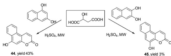
**Scheme 11** Synthesis of benzocoumarins with no substituent at C-4.
