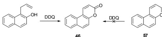
**Scheme 24** Synthesis of benzocoumarin through cyclization followed by oxidation.
