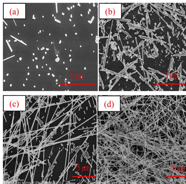
**Fig. 1** SEM images of the silver nanowires prepared with different subsequent reaction time (The time was calculated from the solution turned into a grey emulsion). (a) 0 min; (b) 5 min; (c) 20 min and (d) 30 min.
