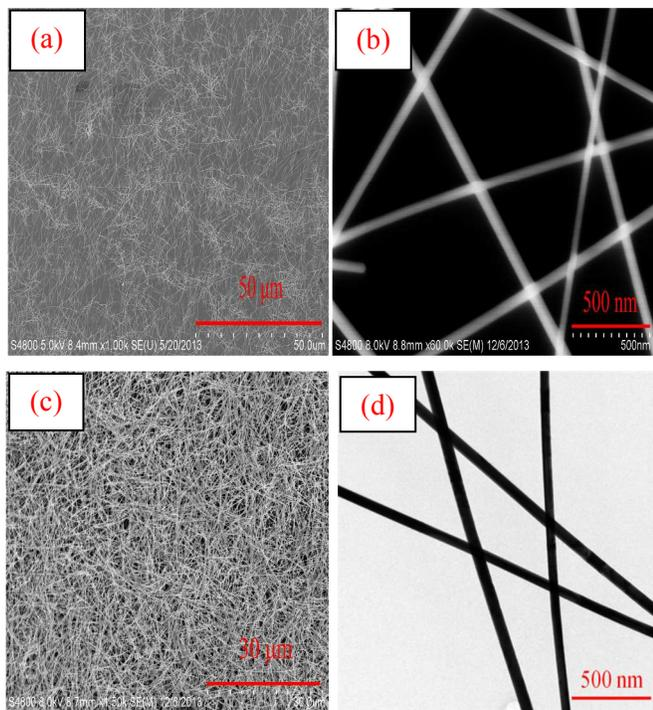
**Fig. 2** Images of silver nanowires prepared with different adding procedure of the subsequent silver nitrate solution: (a) and (b) SEM of the AgNWs prepared *via* successive adding; (c) and (d) SEM and TEM of the AgNWs prepared *via* adding step by step.
