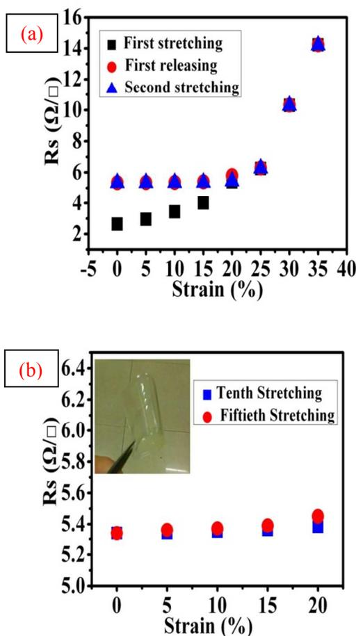
**Fig. 9** (a) Sheet resistance of AgNWs/PDMS as a function of strain. (b) Resistances as a function of tensile strains (0-20%) for the stretchable AgNWs/PDMS electrode in the tenth and fiftieth stretching cycles. The inset is the photograph of AgNWs/PDMS film bent to a small curvature.
