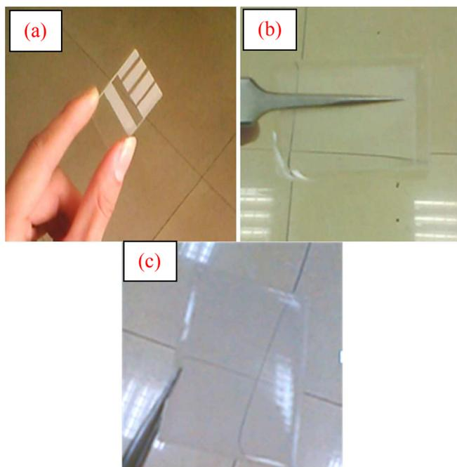
**Fig. 5** Transparent electrodes with different patterns, sheet resistance and transmittance: (a)  $R_s = 2 \Omega/\square$ ,  $T = 62\%$ ; (b)  $R_s = 9 \Omega/\square$ ,  $T = 81\%$ ; and (c)  $R_s = 14 \Omega/\square$ ,  $T = 90\%$ .
