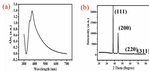
**Fig. 3** (a) UV-vis spectrum and (b) X-Ray diffraction spectrum of the as-prepared silver nanowires.
