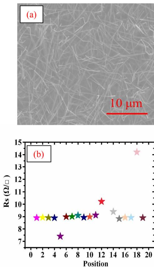
**Fig. 7** (a) SEM image of the AgNWs/PDMS surface morphology; (b) Sheet resistance measured at randomly selected positions.
