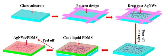
**Fig. 4** The fabrication process of AgNWs/PDMS transparent electrodes.
