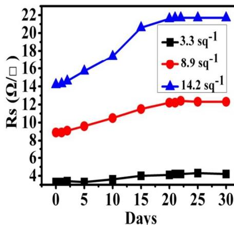
**Fig. 10** Oxidation resistant test. The plot of the sheet resistances versus time for the three AgNWs/PDMS electrodes with different sheet resistances.
