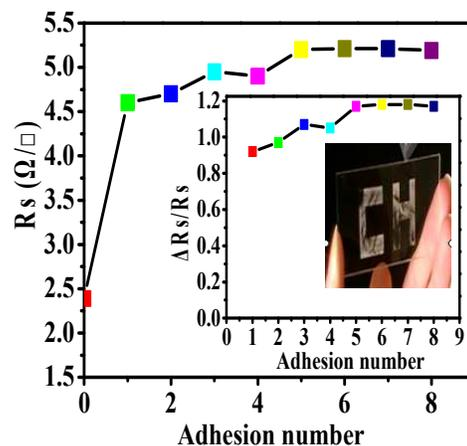
**Fig. 8** Sheet resistance of AgNWs/PDMS transparent electrodes versus adhesion times. The inset is the graph of the relative variation of the sheet resistance versus adhesion times of the resulting AgNWs/PDMS electrode. The image in the inset is the photograph of a transparent electrode prepared by depositing AgNWs to glass substrate directly. After friction, the conductive layer was removed and damaged obviously.
