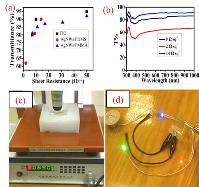
**Fig. 6** (a)  $T\%$  versus sheet resistance of the as-prepared AgNWs/PDMS electrodes and the previously reported comparison data; (b) wavelength versus transmittance graph of AgNWs/PDMS transparent electrodes with different sheet resistance; (c) sheet resistance of the transparent electrodes ( $T = 81\%$ ) measured by four-point probe instrument; (d) flexible transparent conductive film ( $T = 90\%$ ) in an electrical circuit powering three LEDs.
