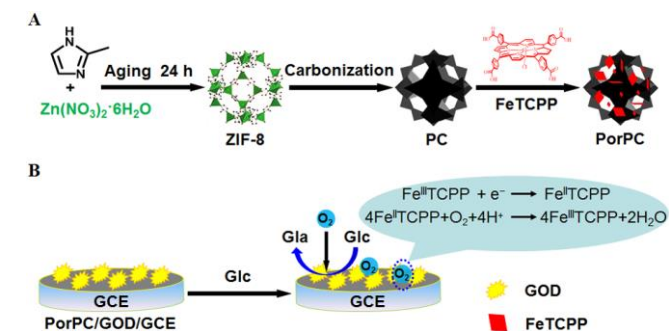
Scheme 1 Schematic representation of (A) preparation of PorPC and (B) sensing mechanism for electrochemical detection of glucose.
