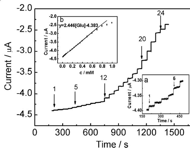
Figure 7 Amperometric response of GOx/PANI microtubes modified GCE to successive addition of glucose in air-saturated PBS (0.1 M, pH = 5.5) at applied potential of -0.5 V. The concentration of glucose: (1) 4.0 μM; (5) 24.0 μM; (12) 0.11 mM; (20) 0.49 mM; (24) 0.89 mM. Inset: (a) Magnification curve with the addition of low concentration glucose from 4.0 to 36.0 μM. (b) The calibration curve of current vs. glucose concentration.
