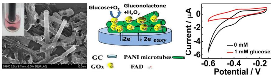
A polyaniline microtubes platform was fabricated for direct electron transfer of glucose oxidase and biosensing applications
