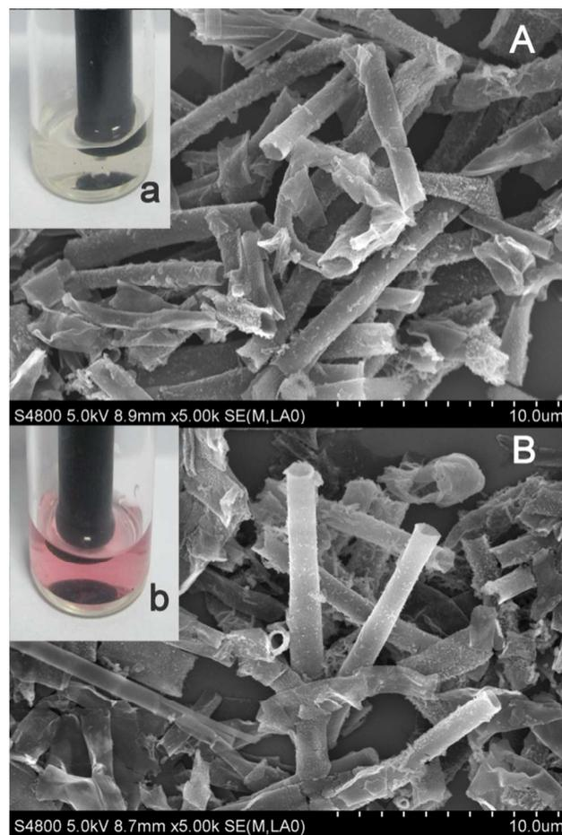
Figure 2 SEM images of PANI microtubes (A) and GOx/PANI microtubes (B). Insets show PANI microtubes modified GCE without (a) or with (b) immobilized GOx in a color system. The concentration of glucose is 5.0 mM. Color reaction time is 30 min.
