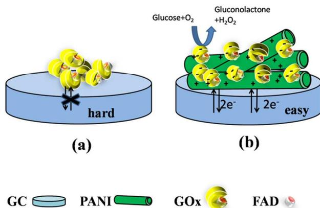
35 Figure 1 Schematic illustration of direct electron transfer of GOx on GCE with or without PANI microtubes.
