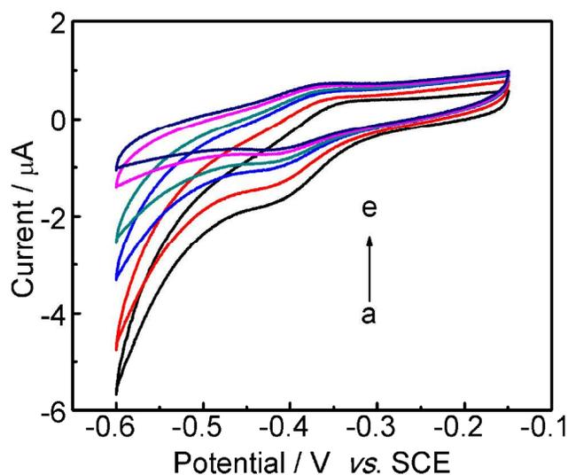
Figure 6 CVs of GOx/PANI microtubes/GCE glucose with various glucose concentration of 0 mM (a), 0.2 mM (b), 0.4 mM (c), 0.6 mM (d) and 1.0 mM (e) in air-saturated PBS (0.1 M, pH = 5.5).
