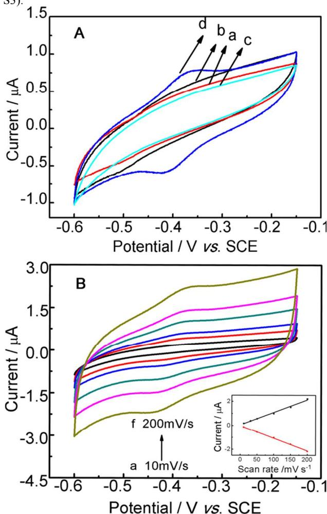
Figure 4 (A) CVs of bare GCE (a), PANI microtubes/GCE (b), GOx/GCE (c) and GOx/PANI microtubes/GCE (d) in oxygen-free PBS (0.1 M, pH = 5.5) at the scan rate of 100 mV/s. (B) CVs of GOx/PANI microtubes modified GCE in oxygen-free PBS at different scan rate. Scan rate (a-f): 10, 30, 50, 100, 150, 200 mV/s. Inset: the plot of anodic and cathodic peak current vs. scan rates.
