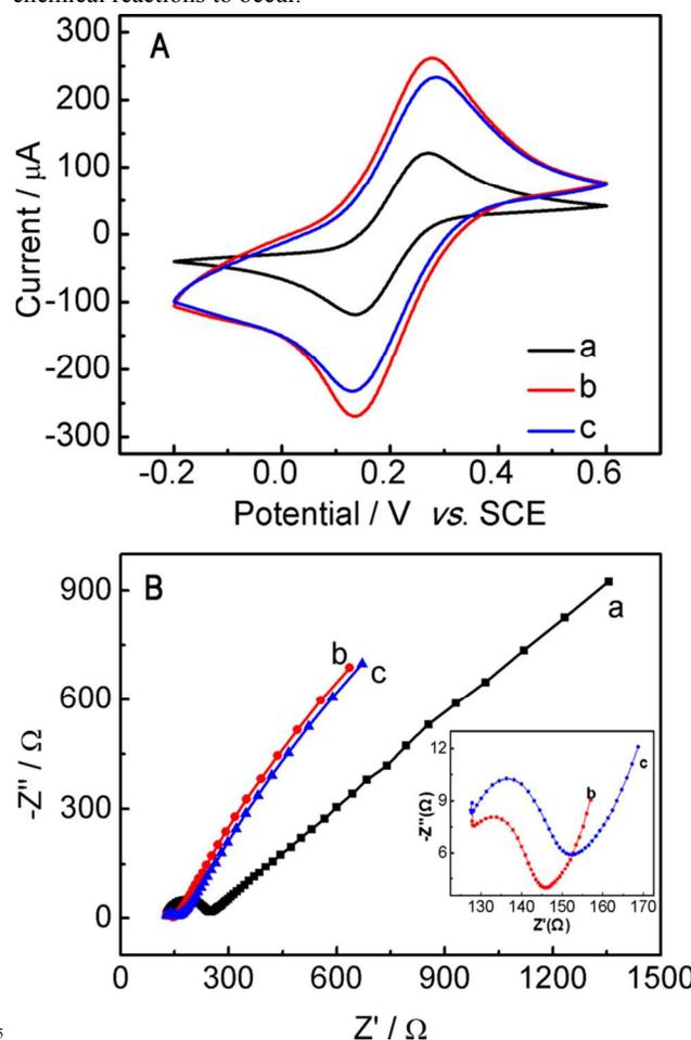
Figure 3 (A) CVs of bare GCE (a), PANI microtubes/GCE (b), and GOx/PANI microtubes/GCE (c) (B) EIS of bare GCE (a), PANI microtubes/GCE (b), and GOx/PANI microtubes/GCE (c) in 10 mM  $\text{Fe}(\text{CN})_6^{3-/4-}$  with 0.1 M KCl supporting electrolyte.
