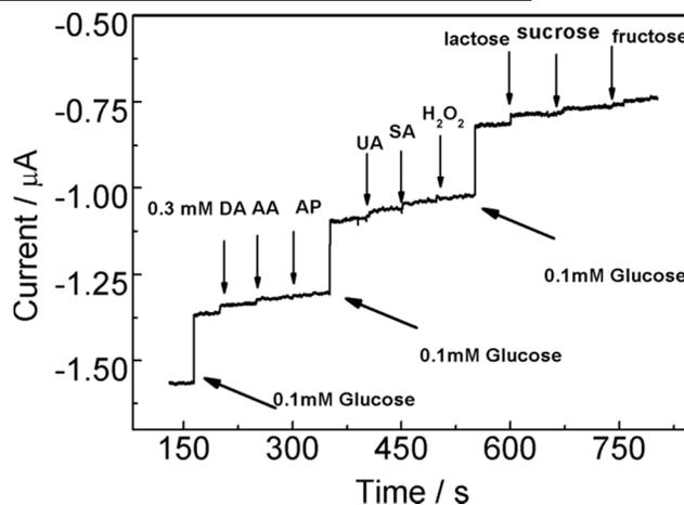
Figure 8 Amperometric response of the GOx/PANI microtubes/GCE to the addition of 0.1 mM glucose or 0.3 mM other interferences in 0.1 M air-saturated PBS at the potential of -0.5 V.
