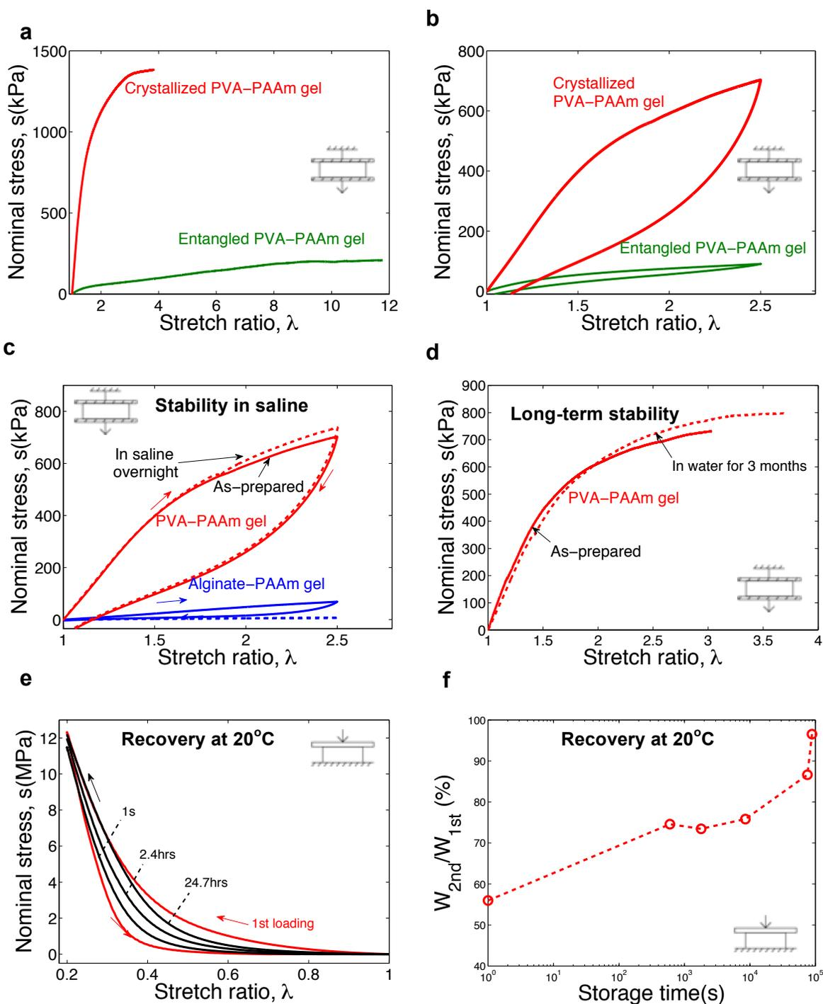
**Figure 2. Crystallites as stable and recoverable cross-links.** **a**, Stress-stretch curves of two types of gels. Each sample is stretched to rupture. The nominal stress is the applied force divided by the cross-sectional area of the undeformed sample. The stretch ratio is the length of deformed sample divided by the initial length. **b**, Loading-unloading curves of both gels. Each sample is
