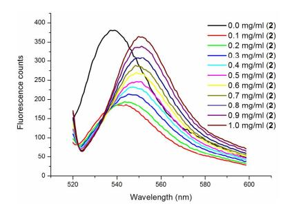
Figure 3. Emission spectra of eosin (10  $\mu$ M) recorded with increasing concentration of Pep-Neo (2)
