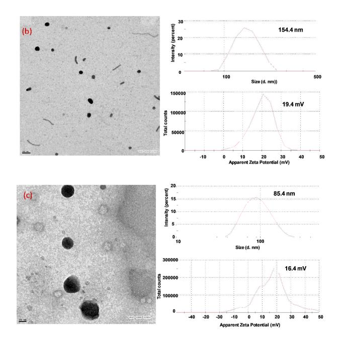
**Figure 2.** TEM images of (a) Pep-Neo (in  $H_2O$ ), scale bar: 0.2 µm, (b) Pep-Neo/pDNA complex (at w/w ratio of 66.6 in  $H_2O$ ), scale bar: 100 nm, and (c) Curcumin-entrapped Pep-Neo nanostructures, scale bar: 20 nm.
