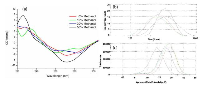
**Figure 4.** (a) CD spectra of Pep-Neo nanostructures in different composition of methanol/water, (b) and (c) change in the size and zeta potential of nanostructures with increasing methanol percentage in water, respectively.
