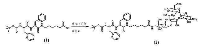
**Scheme 1.** Schematic representation of synthesis of Pep-Neo (2). *Reaction conditions: (a) NMM/IBCF, (b) NHS, and (c) Neomycin sulfate /Na*<sub>2</sub>CO<sub>3</sub>
