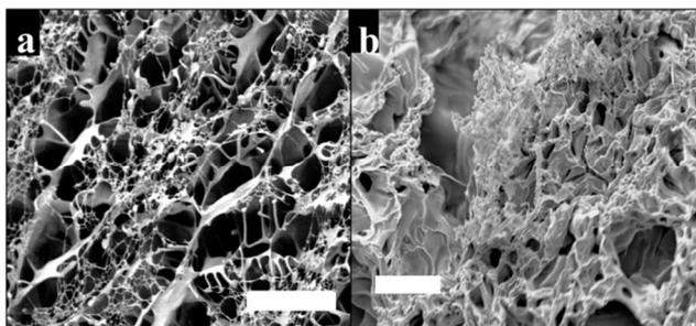
Figure 6, SEM images of freeze dried 2-UArg-2-S/F127-DA/alginate (1:4, w/w) hybrid hydrogel (a: 0 day incubation in PBS; b: 30 days incubation in PBS). White scale bar is 30  $\mu$ m.
