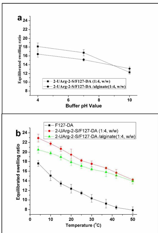
Figure 3, Equilibrium swelling ratios of the hybrid hydrogels in aqueous solution as a function of the pH value (a, at room temperature) and temperature value (b, in DI water)
