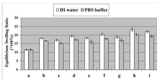
Figure 2, Equilibrated swelling ratio of Arg-UPEA/Pluronic-DA/alginate hydrogels in PBS (pH=7.4) solution and DI water at room temperature. a) Pure F127-DA hydrogel (control); b) 2-U-Arg-2-S/F127-DA (1/4, w/w); c) 2-U-Arg-2-S/F127-DA/alginate (1/4, w/w); d) 2-U-Arg-4-S/F127-DA (1/4, w/w); e) 2-U-Arg-4-S/F127-DA/alginate (1/4, w/w); f) 2-U-Arg-2-S/F127-DA (2/3, w/w); g) 2-U-Arg-2-S/F127-DA/alginate (2/3, w/w); h) 2-U-Arg-4-S/F127-DA (2/3, w/w); i) 2-U-Arg-4-S/F127-DA/alginate (2/3, w/w)
