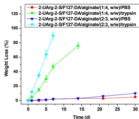
Figure 5, Biodegradation of the Arg-UPEA/Pluronic-DA/alginate hydrogel at 37 °C
