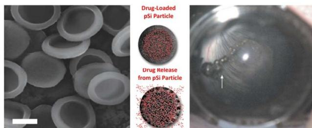
**Fig. 8** SEM image of porous silicon microparticles produced by lithography combined with electrochemical etching (scale bar = 1  $\mu\text{m}$ ), schematic diagram showing how these particles load and release drug (adapted from Ref. [165]) and surgical microscope image obtained immediately after intravitreal injection of fresh pSi microparticles in the vitreous cavity (arrow) of a New Zealand Red rabbit (adapted from Ref. [159]).
