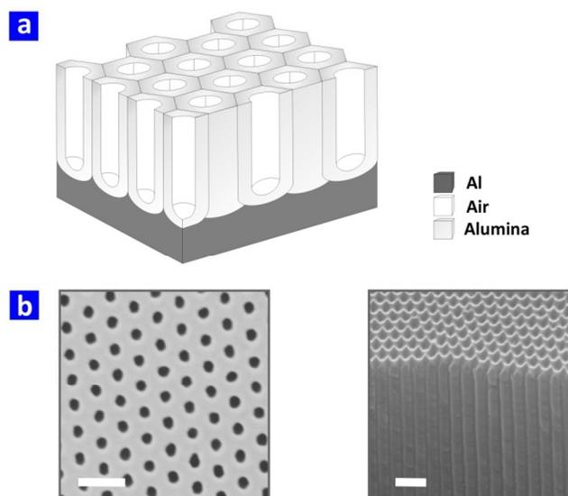
**Fig. 3** Use of NAA for developing drug-releasing implants. a) Schematic illustration of the basic structure of NAA. b) Top and cross-section scanning electron microscopy (SEM) images of NAA (scale bars = 400 and 250 nm, respectively).
