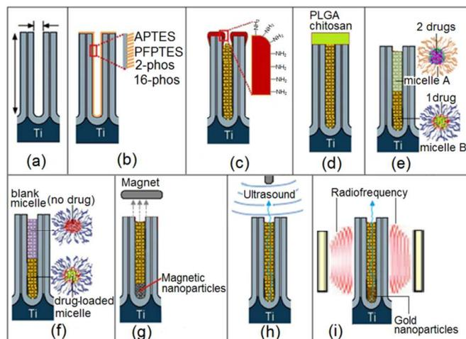
**Fig. 6** Schematic diagram showing different strategies developed by our group for controlling drug release from drug-releasing implants based on TNTs (adapted from Ref. [98]).
