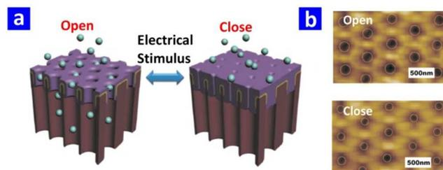
**Fig. 4** Electrically responsive drug-releasing NAA chip (adapted from Ref. [100]). a) Schematic diagram showing the mechanism of an electrically responsive drug-releasing chip based on NAA and PPy-DBS (reversible cycle). b) Atomic force microscopy (AFM) images of these NAA chips before and after the application of voltage (pore mouth reduction).
