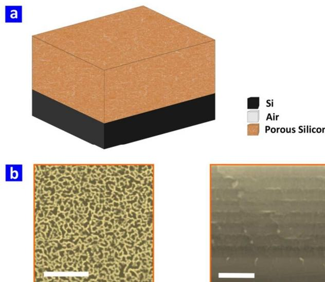
**Fig. 7** Use of pSi for developing drug-releasing implants. a) Schematic illustration of the basic structure of pSi. b) Top and cross-section scanning electron microscopy (SEM) images of pSi (scale bars = 200 and 2.5  $\mu\text{m}$ , respectively).
