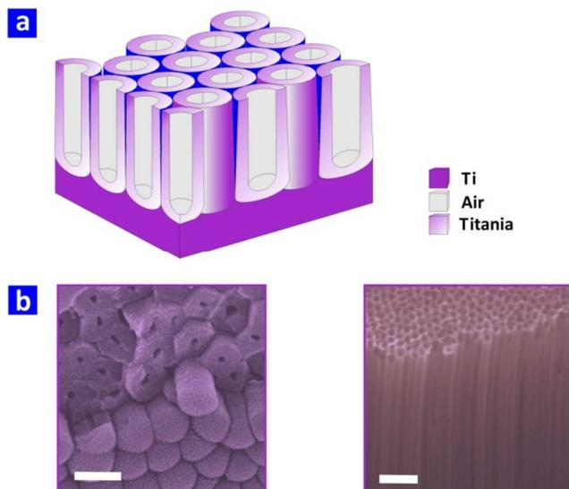
**Fig. 5** Use of TNTs for developing drug-releasing implants. a) Schematic illustration of the basic structure of TNTs. b) Top and cross-section scanning electron microscopy (SEM) images of TNTs (scale bars = 100 and 500 nm, respectively) (adapted from Ref. [118]).
