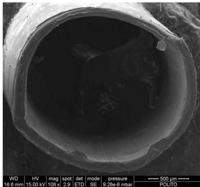
Figure 9. SEM images of a fractured section of a PU guide. Nerve guide was produced by melt-extrusion from a biocompatible novel polymer: a synthesized poly(ester urethane) having PCL as macrodiol and two commercial molecules as chain extender and linker (CDM and HDI, respectively).
