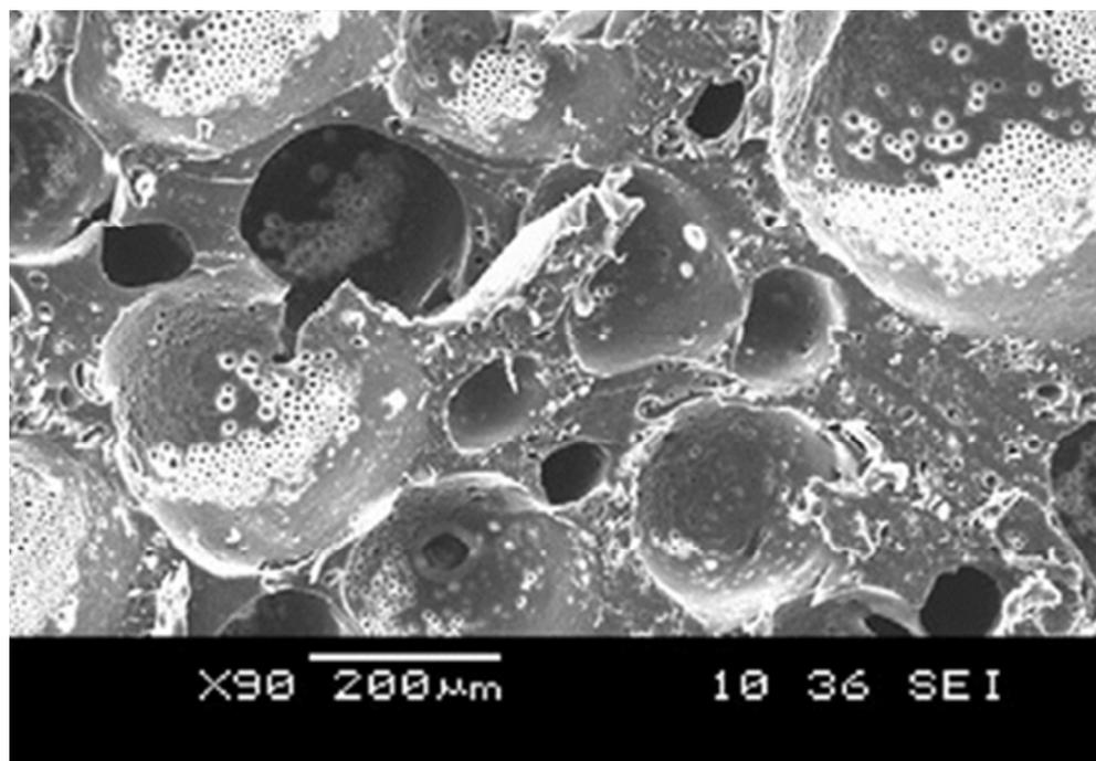
Figure 4. Fractured section of a PU/HA (1% HA) adhesive material. Reprinted with permission.<sup>39</sup> Copyright © 2012 Wiley Periodicals, Inc
