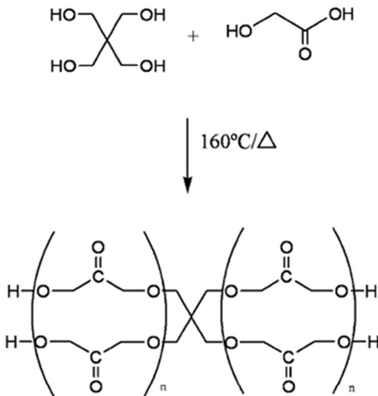
Figure 6. Schematic representation of the synthesis of prepolymer B: condensation reaction. Reprinted with permission.<sup>46</sup> Copyright 2007, Elsevier.
