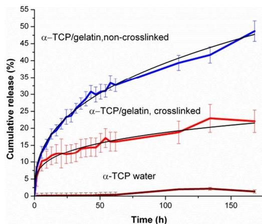
**Figure 6.** Cumulative release of gelatine during setting for the non-crosslinked (blue) and crosslinked (red) samples, together with the reference material without gelatine (brown). The black line corresponds to the data fitting with the Korsemyer-Peppas model (eq. 2).
