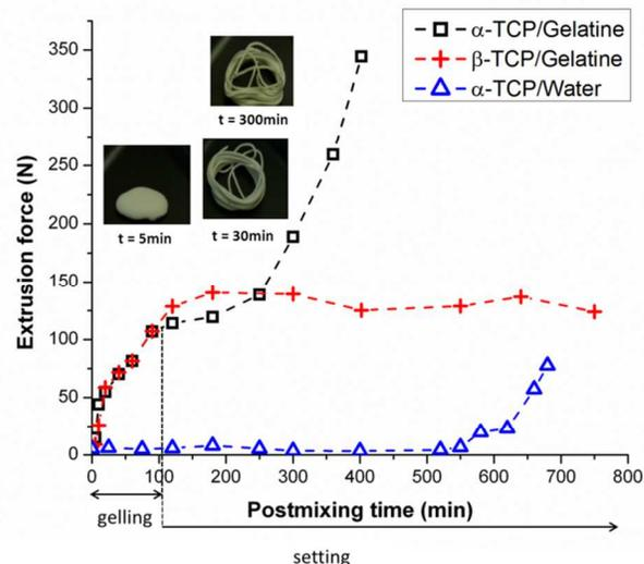
**Figure 1.** Mean extrusion force of reactive ( $\alpha$ -TCP) and non-reactive ( $\beta$ -TCP) inks as a function of post-mixing time. Inks were prepared either with or without gelatine. Insert pictures show the aspect of the extruded material at three different post-mixing times. The standard deviation for each time point were too small to be properly represented.
