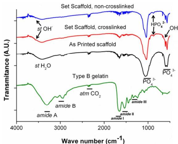
**Figure 5.** FTIR spectra of pure gelatine (green), as printed scaffold (black), set crosslinked scaffold (red) and set non-crosslinked scaffold (blue). The intensity of the characteristic amide stretch bands and vibrations of gelatine (A, B; I, II, III,) decreased upon setting, more markedly in the non-crosslinked scaffold. Furthermore, the characteristic bands for OH<sup>-</sup> and HPO<sub>4</sub><sup>-</sup> of CDHA were detected in the set scaffolds.
