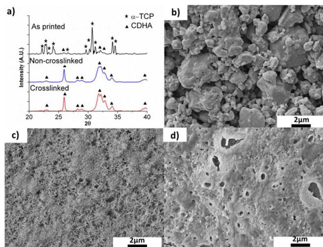
**Figure 4.** a) X-ray diffraction patterns of as printed (black) and set robocasted scaffolds (7 days of setting), both non-crosslinked (blue) and crosslinked (red). Stars and squares represent the reference diffraction patterns of  $\alpha$ -TCP and CDHA, respectively. Indexed diffractograms are provided in the Supplementary Information (Figure S2).; SEM micrographs of the surface of the strands in the scaffolds are shown in b) as printed, c) non-crosslinked, and d) crosslinked set scaffolds.
