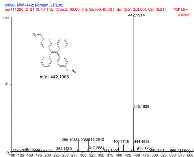
Fig. 1 High resolution mass spectrum of TPE-2N<sub>3</sub>.
