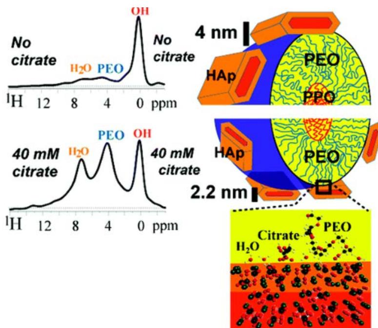
Figure 10. Nanocomposite formed by HAp nanocrystals precipitates on the self-assembled PEO-PPO block copolymers. NMR spectra showed that higher citrate concentration will reduced the size of HAp nanocrystal (reprinted with permission from reference 5).<sup>5</sup>
