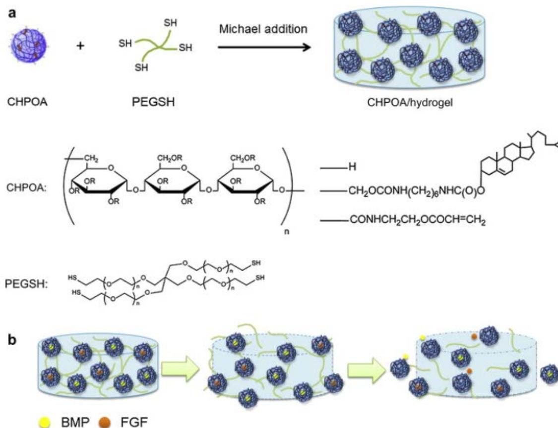
Figure 9. (a) Synthesis of the CHPOA/PEG-SH hydrogel and their chemical structure. (b) Releasing of the FGF18 and BMP2 as the hydrogel degrades. (reprinted with permission from reference 184).<sup>184</sup>
