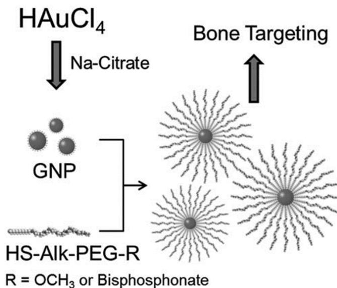
Figure 4. AuNPs modified with heterobifunctional PEG derivatives bone mineral targeting (reprinted with permission from reference 116).<sup>116</sup>
