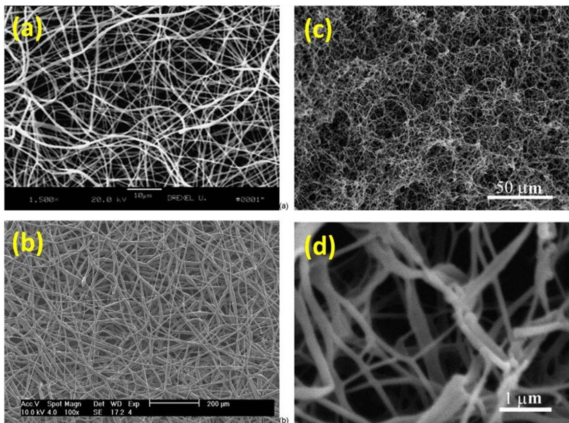
Figure 7. SEM micrographs of nano-fibrous scaffolds for bone tissue engineering. (a) the electrospun PLGA nano-fibrous structure. (b) electrospun PCL scaffolds. (c) and (d) a PLA fibrous matrix prepared by phase separation technique. (c) 500 $\times$  and (d) 20K $\times$  (reprinted with permission from reference 165).<sup>165</sup>
