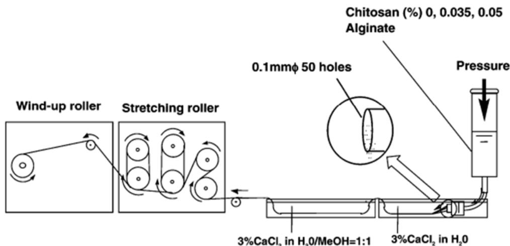
Figure 15. The spinning process of alginate fiber coated with chitosan (reprinted with permission from reference 209).<sup>209</sup>
