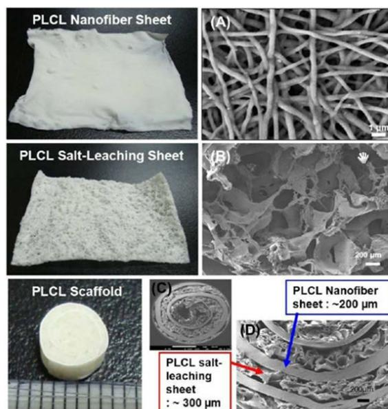
Figure 16. SEM images and photographs of PLCL scaffolds. PLCL nanofiber sheet by electrospinning(A), followed salt-leaching (B), PLCL scaffold by rolling (5 mm in diameter and 3 mm in thickness in left section) (C) and PLCL scaffold with a high magnification(D) (reprinted with permission from reference 225).<sup>225</sup>
