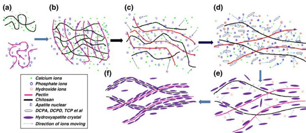
Figure 3. Schematic model of nano-HAp crystals synthesis process in the presence of chitosan–pectin PECs network. (reprinted with permission from reference 86).<sup>86</sup>
