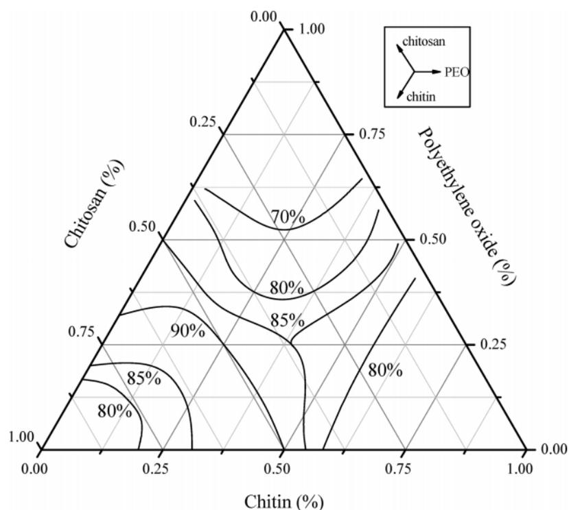
Figure 13. Porosity changes of the chitosan/PEO/chitin scaffolds in ternary phase diagrams. Note: the data were calculated by mean value of all compositions ( $n=3$ ), and the axes indicated the weight percentage of the various components (reprinted with permission from reference 208).<sup>208</sup>
