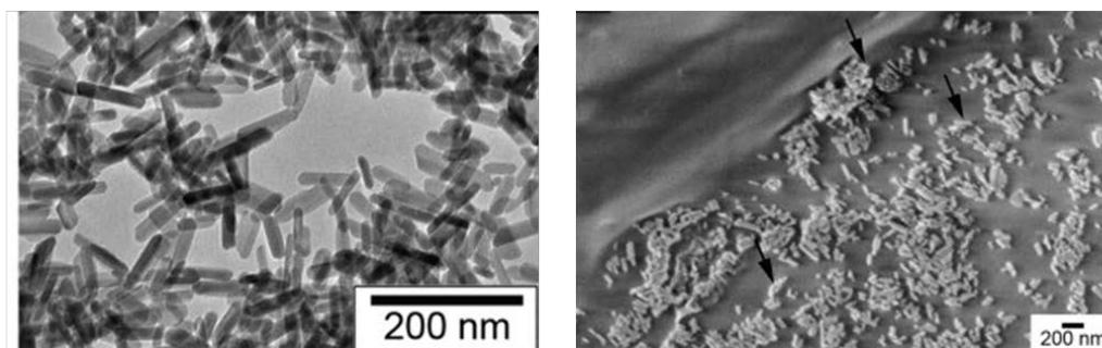
Figure 8. A two-step HAp nanoparticle synthesis process. TEM images (bottom left) of the HAp nanoparticles used to prepare mineral-containing scaffolds. SEM image (bottom right) showing the HAp nanoparticles on the scaffold surface, and arrows point to individual particles (reprinted with permission from reference 171).<sup>171</sup>
